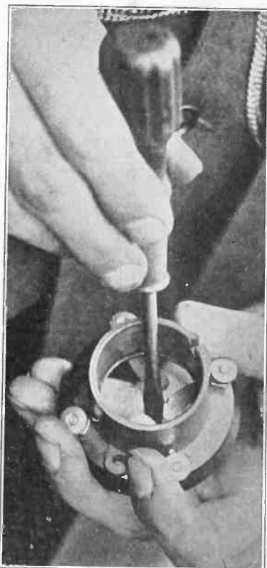
STATIC? No! Bad B batteries? No! A loose wire? No! Yet the noise and crackling persists. Look to your sockets. See that the contact is firm and clean. Use the screw-driver, as shown, to bend to contact springs so as to make the connection on the tube more permanent. (Kadel & Herbert.)
