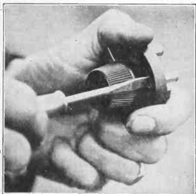
HERE is a potential location of noise. When putting your set together be sure that every connection is tight, and when examining the various parts, don't overlook the rheostat. (Kadel & Herbert.)
