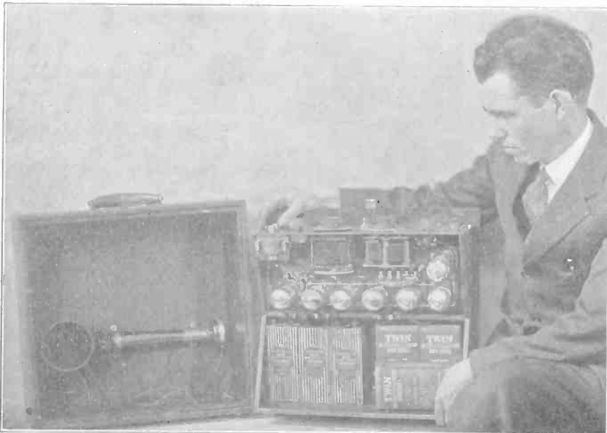
PACIFIC coast stations have been heard in Washington, D. C., on this 7-tube portable Super-Heterodyne. It is wholly self-contained. Brent Daniel, formerly an engineer of the Bureau of Standards, has the honor of being the one who built it. (Harris & Ewig.)
