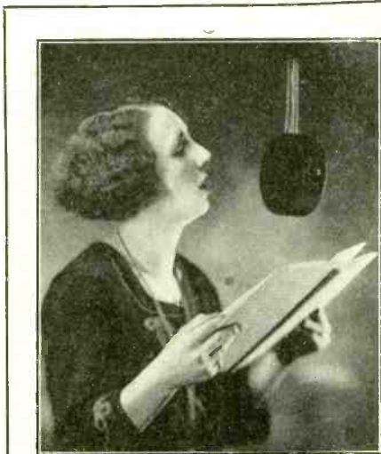
Singing into the new Thomas "glow" transmitter at Station KDKA. This transmitter has no diaphragm and is said to give perfect sound reproduction.
