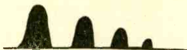
Figure 2. After passing through detector, wave of Figure 1 has been reduced to this form. The negative wave has been strained out by the crystal.
