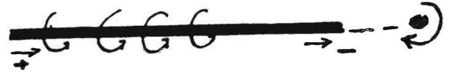
Figure 3—If you grasp the wire with your thumb pointing in the direction of the flow of the current, your fingers will follow the direction taken by the lines of force surrounding the wire.
