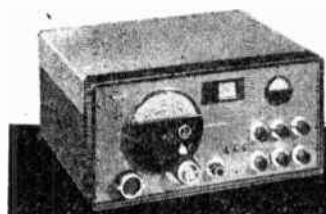
Hallicrafters new Model SX-42 covers from 540 kc. to 110 Mc., AM, FM, CW
