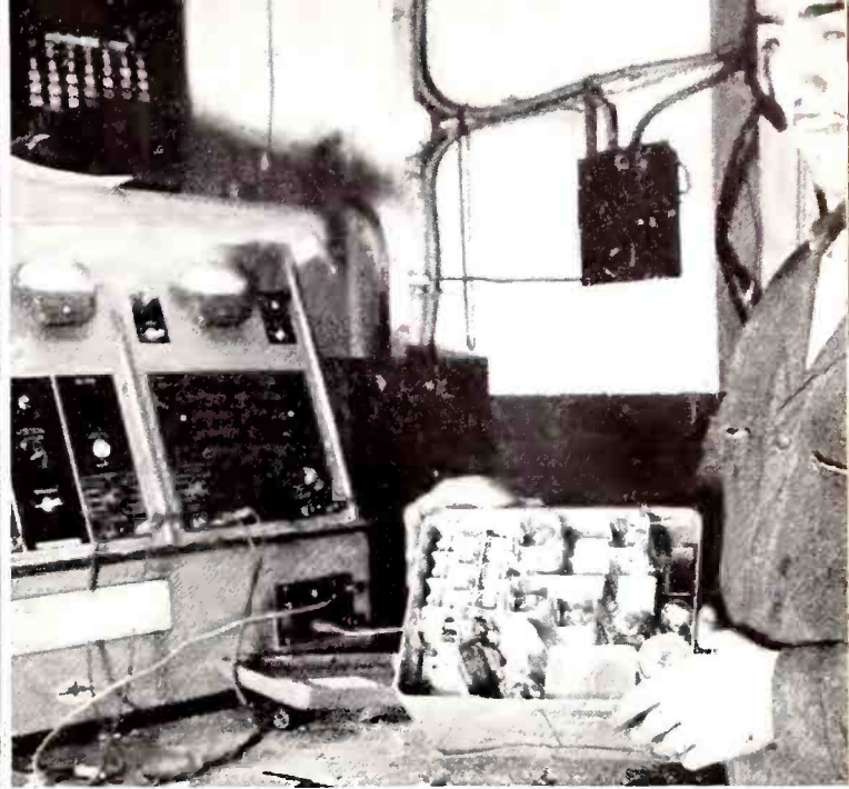
4. Dead sets are pulled out of car after preliminary check shows antenna and power to set OK. Service bench outlets provide speaker and battery connections for test.
