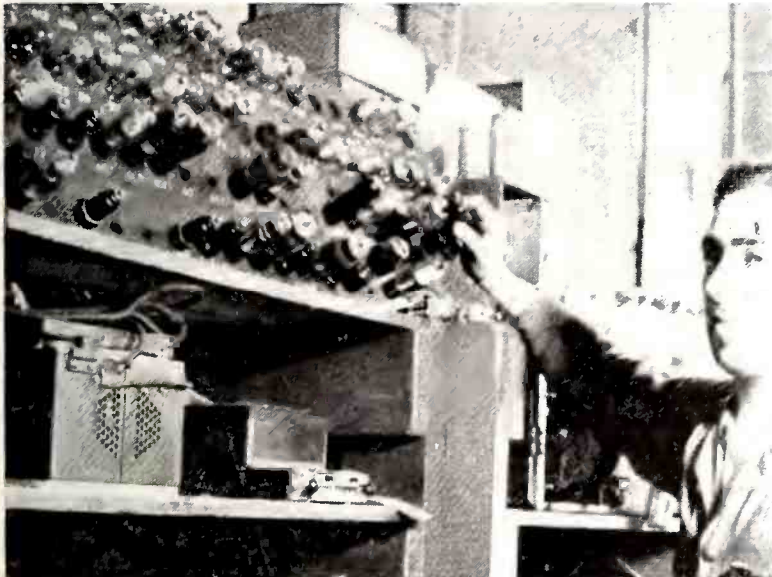
3. Every job involves its own contortion act. Here the T-bolts were put through bulkhead and nuts partly threaded on. Chassis was then hooked over the bolt heads. Bolts then pulled up in position and nuts spun tight, not "worked" on.
