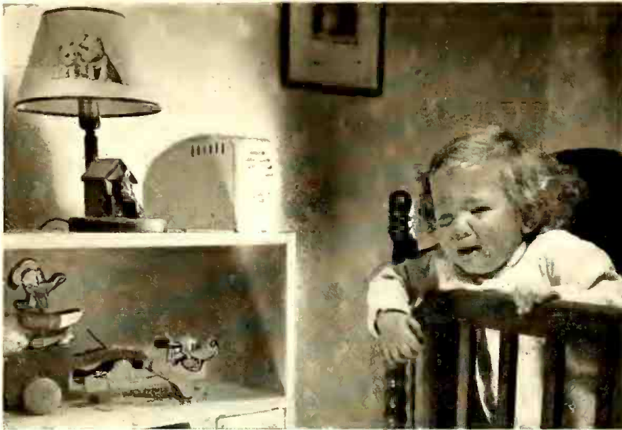
Here is the "Guardian Ear" unit of Zenith's new wireless "Radio Nurse." Plugged into the nearest outlet, it reports everything to "voice" unit in another room.
