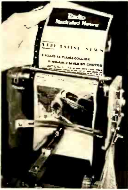
Broadcasters and public are all getting excited about facsimile. Here's the Finch home printer, for attachment to any radio.
