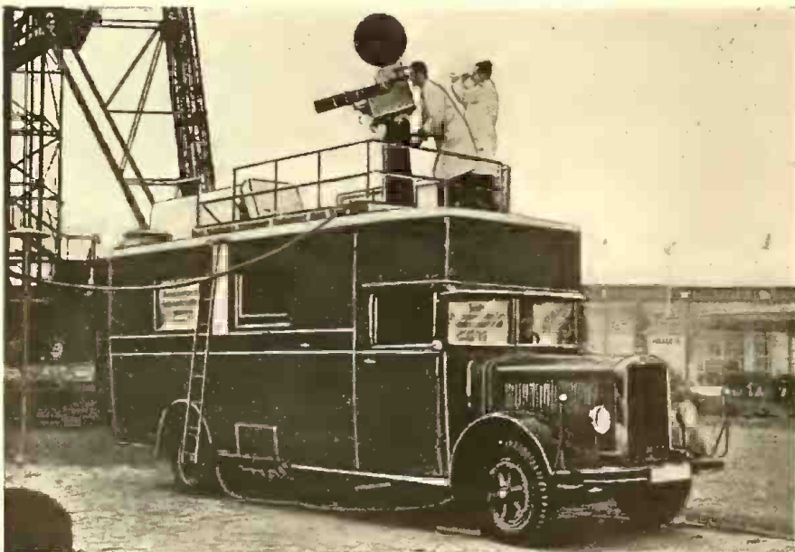
Television-camera truck in Berlin, Germany. Motion-picture film as exposed is fed down into truck-body to be developed and then scanned for transmission on television circuits, with less than half a minute delay.
