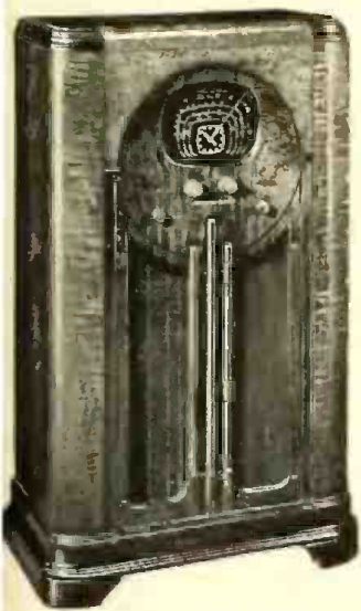
MODEL 670C —"Automatic Maestro" model; 9 tube, 11 tube performance, All-Wave American, Police and Foreign, plus U. S. weather band, improved superheterodyne Console. Range: standard broadcast and police 525 to 1800 Kilocycles; police and short wave 1800 to 6000 Kilocycles; and long wave U. S. weather band 150 to 375 Kilocycles.
