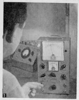
Determining leakage current at various collector voltages. Transistor under test is in socket at right of large meter.
