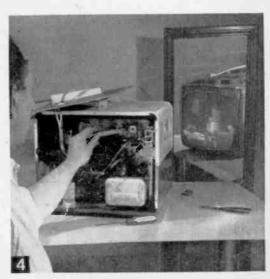
The service tech uses an insulated plastic wand to tap tubes. He watches the screen in a mirror, or reflected from a window. Erratic picture or sound pinpoints the faulty tube.
