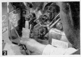
Every set has a tube layout, either a decal or sticker fastened somewhere on the inside wall or chassis. Do not remove chassis or tamper with picture tube adjustments. You may need a Photofact folder (see text).
