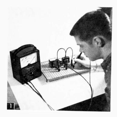
Simple 11-step power supply offers a variety of voltages to operate tube heaters, test intermittent equipment, correct line current and handle other applications
