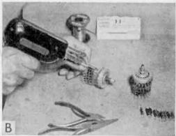
Shape resistor leads around two nalls driven in a block of wood to get them of uniform length and with uniform loops (A); then, starting with terminal #1 on each switch with the lowest value resistor, position looped ends of resistors and solder at each terminal (B).
