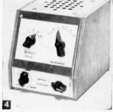
On the seconds range, you get a click every 1, 5, 10, 30, or 60 seconds. Each range has its own control pot on the back of the chassis for calibration.
