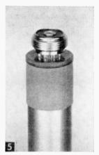
Insulated installation of connector, ready for any standard mike.
