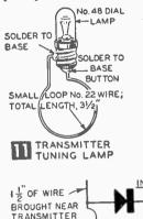
of the transmitter 25 mmf antenna tuning capacitor and a twisted pair of wires run to the 0-to-1 milliammeter on the front of the chassis. Apply power, and throw send-receive switch to send. If the meter reads backwards, reverse the leads to it. Position the pickup lead so that when
