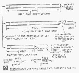
close to a TV channel frequency that an antenna filter might also filter out the desired signal, connect a simple filter or trap to the antenna terminals of the TV set (with the regular antenna lead). If you know the TVI frequency, make the filter of a section of 300-ohm antenna lead-in cut to exactly 1/2 the wavelength of that signal as in Fig. 9; solder the free ends of the stub together. If you don't know the TVI frequency, cut the
