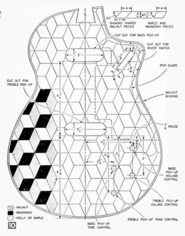
The sub-top and sub-back (Fig. 4) are next on the agenda. Although the original guitar has the inlaid cubic design on both the top and the back, you may wish to inlay the top only, in which case you need not make a sub-back. Instead, substitute the sub-back with inlay, with a single piece of  $\frac{1}{8}$  in. thick maple plywood.
