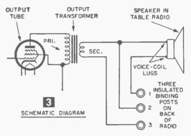
How to Wire. Fig. 1 shows the installation on an FM table radio; Figs. 2 and 3 furnish the wiring info. Do not disturb the two wire leads, usually red and blue, on the primary side of the output transformer. If you cannot find a place for the posts on the rear panel where they won't interfere with the loop antenna, if any, mount the posts on a strip of insulating material and fasten with an angle bracket to the back of the cabinet.
