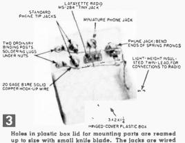
in parallel, with solid copper hook-up wire.
