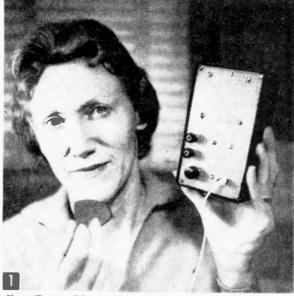
The utility amplifier can be used with a microphone as above or as a voltmeter audio amplifier.
