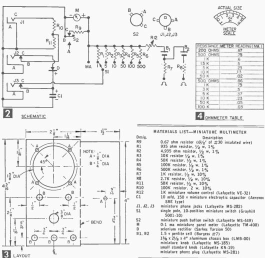
the rubber cement handy, cut out and fasten the meter scale (Fig. 4) on the front of the meter glass.
