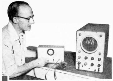
Oscillogram pattern of a full-wave, battery charger rectifier showing lower halfcycle, (lost in Fig. 4) inverted and above horizontal centerline, indicating it is being used.
