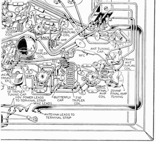
the receiver throughout its range. At some point on the dial the hiss should disappear. Turning the grid-dip meter off should cause it to reappear. If it does, the receiver is operative. If it doesn't, you'll need to recheck the wiring in the mixer and R.F. amplifier circuits only; the oscillator has been checked.
