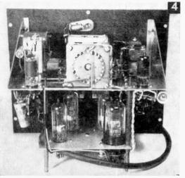
Back view of unit showing dual chassis construction.
