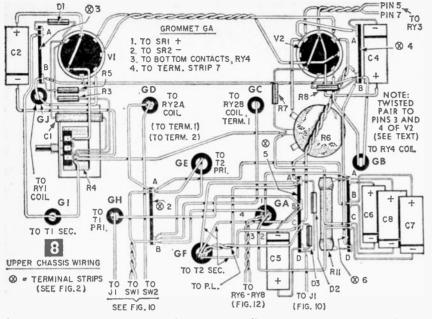
the two chassis (which rest on the bottom) will properly support the upper chassis. If scrap aluminum is not on hand, a  $3\frac{1}{2} \times 6 \times 8$ -in. "Minibox" (Bud CU-3009 or CU-2109) will provide all that is required. The flanged side of this box will make the upper chassis merely by cutting the ends of the box to make the side supports, and the other half of the box will make the lower chassis and the 2 x 2-in. mounting for R4.
