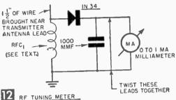
the transmitter is operating and the antenna is properly loaded the meter reads about mid-scale. The transmitter may now be easily adjusted by tuning for the greatest meter reading.
