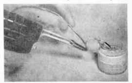
parts while applying solder. Enlarge hole in clip slightly with a drill and attach to can with a small relf-tapping metal screw.—JOHN A. COMSTOCK.
