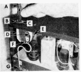
(A) Steel rule, (B) fiber washer, (C) bolts, (D) friction tape,
