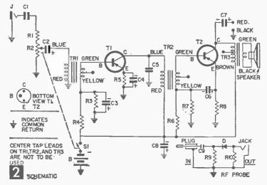
the collector of T2 to an output terminal. An ac voltmeter or an oscilloscope may be connected from this terminal to monitor the output voltage of the amplifier.
