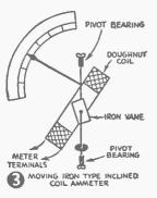
have powerful magnets, they often accumulate bits of iron or steel and these often introduce frictional factors. Their removal may usually be effected with the sharpened end of a paper clip. One must make sure, however, that all metal filings are removed from the end of the paper clip wire before it is introduced into the
