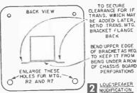
type speaker permits direct drive. Although this arrangement results in a comparatively low efficiency output impedance match, it eliminates the need for a space-consuming transformer or a miniature transformer which would compromise the frequency response and result in poor tone.
