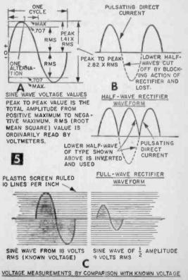
Oscilloscope pattern quickly identifies a half-wave rectifier. Note that lower half wave has been cut off and lost.
