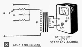
a text explaining how to adjust and use it, how it works, and how to apply the circuit. In addition to this specific information for each circuit, the manual has sections on how radio works, transistors, capacitors and resistor color codes, and electronic symbols.
