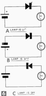
are oppositely connected to the respective lamp bulbs, one—and only one—of the lamps will light, the position of the switch determining which one will. No black magic after all.
