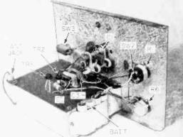
Transistor TRI, a Philco surface-barrier type, is the critical transistor. It is used as a superregenerative detector.
