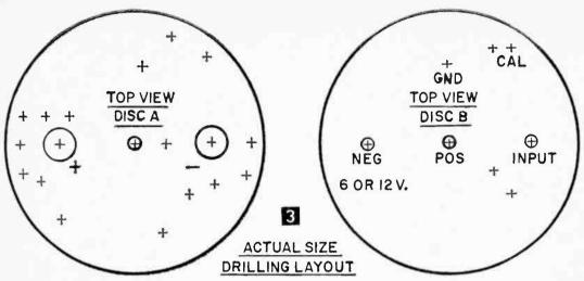
Use a 4-40 screw for the calibration switch S1 (Fig. 3). When all parts are assembled, this switch operates by turning the screw in and out of its threaded hole in Disc B, and it contacts the C4-V1 terminal.
