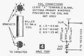
with any capacitor having a maximum capacitance between 250 and 500 mmf.
