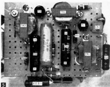
structed in the smallest amount of time if all parts are available when construction is begun (see Materials List), and if this work sequence is followed: 1) Prepare circuit board; 2) prepare panel board; 3) mount components on circuit board; 4) wire circuit board; 5) mount components on panel board; 6) wire panel board; 7) mount circuit board on panel board, and make interconnections.
