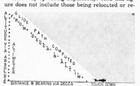
A control system incorporating DECCA—RAILS (Remote Area Instrument Landing System). Although the accuracy of this system is still being evaluated, chances are good it will enhance DECCA's overall superiority. At present it's only commercicl use is in conjunction with the Bell helicopter service in the Dallas-Fort Worth area.
