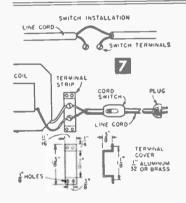
plug cap to the other end. Connect cord to the terminal screws of the terminal strip and make a small clamp to hold cord securely. Place a small cover piece over the live terminals of the terminal strip as protection against accidental shock, screwing through holes in the cover and also down through holes in the terminal strip, to hold the assembly to the base, taking care to
