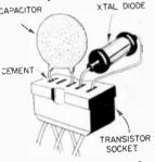
much heat from a soldering iron. Just insert the leads into the socket, then add a touch of service cement to the lead where it enters the socket.
