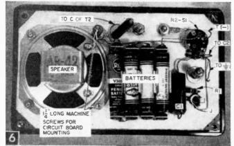
Fasten the knob on the shaft of R2-S1 and turn on to full volume. Touch the tip contact
