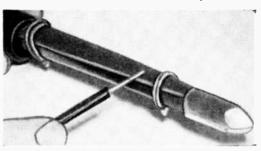
• Quite often a small file is needed to file corroded parts and wires clean before the application of solder. If you want to eliminate the necessity of hunting up such a file every time you have a soldering job to do, attach one to your iron's barrel with heavy solid wire. (You may have to break off the file's tang if it is longer than your iron's barrel.)—J.A.C.
