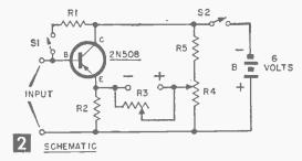
**Construction.** The circuit is shown in Fig. 2. Miniature perforated board layout is shown in Fig. 3. The entire assembly is housed in a plastic case (See Fig. 4). First, prepare the circuit board. The board on the Materials List is the exact size required, the hole centers coincide with perforations. Drill a ¼-in. hole for each hole position (back the board with a wood block to prevent breakage). The larger holes may be made with a taper reamer or with drills of appropriate size.
