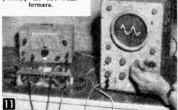
bility open to the owner of an oscilloscope. It is often necessary to determine the frequency of some power source and this can be done quite easily by what are known as Lissajous figures. By this method a known frequency is applied to the horizontal channel and the unknown to the vertical channel to produce a variety of patterns that can be interpreted to indicate the frequency of the unknown signal. Fig. 9 shows some of the Lissajous patterns obtained.
