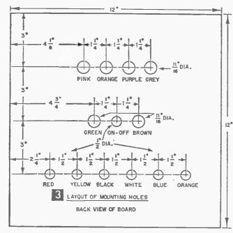
The switches, unlike the lamp sockets, mount vertically. This will place the "o" terminals on the top and the "c" terminals on the bottom, the "1" switch on the left, and the "2" switch on the right.
