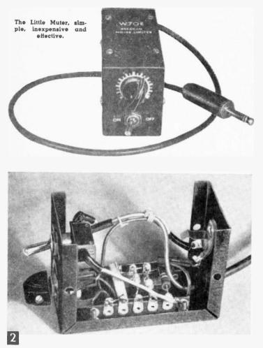
Internal view of noise limiter showing component mounting on tie points.
