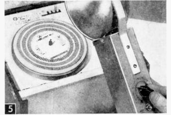
An ordinary record turntable and stroboscopic disc are used to calibrate your strobe light.
