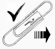
Nestled inside this paper clip—with room to spare—is a tunnel diode, one of last year's most startling electronics developments. If an FM receiver were rebuilt using one of the new diodes, all the conventional components shown at the right could be omitted.
