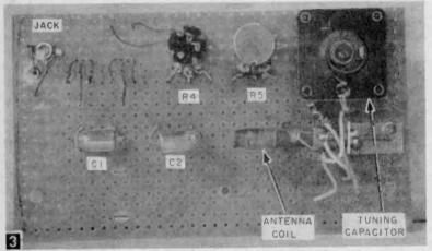
Back view of home-made lab kit circuit board.
