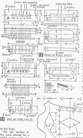
of six  $\frac{1}{4}$  in. dia. magnets  $1\frac{1}{4}$  in. long by inserting the magnets through the  $\frac{1}{4}$  in. holes. Cement magnets in place with household cement.
