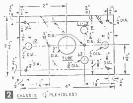
jacks, J1 and J2, are not shown and should be positioned for the particular sized component used;  $\frac{1}{8} \times \frac{1}{4}$ -in. machine screws mount all parts. By using a 3/32-in. hole, the screws will tap themselves into the soft Plexiglas. The four  $\frac{1}{8}$ -in. holes are for mounting the chassis to its cabinet with  $\frac{1}{8} \times \frac{1}{2}$ -in. screws.
