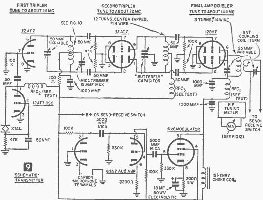
just the first-tripler 50 mmf tuning capacitor until the tuning lamp (still in the second-tripler circuit) glows brightly. Now, adjust the first-tripler 15 mmf mica trimmer capacitor and the first-tripler 50 mmf tuning capacitor alternately, until the tuning lamp glows at nearly full brilliance.
