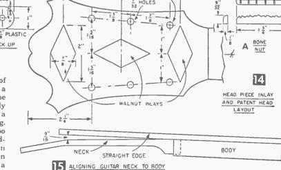
the neck should be a slight angle with the top surface of the body when tested with a straightedge as in Fig. 15. If you file away too much stock, use wooden shims to fill in where needed. When you are satisfied with a good fit, glue the neck
