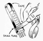
around the bottom with another strip of tape. Don't use tape on tubes that heat up excessively, because of the possible danger of fire due to tape igniting. *Never* use plastic tape for this purpose as it ignites easily.—J. A. COMSTOCK.
