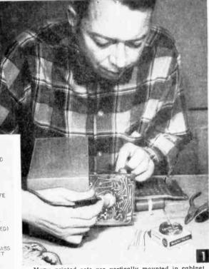
Many printed sets are vertically mounted in cabinet and slide out for quick circuit repair. Note that a fine-tip pencil iron, not over 40 watts, is used to prevent wiring damage.
