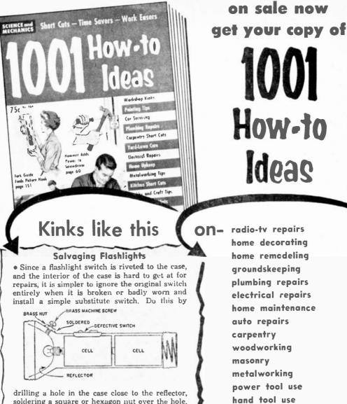
soldering a square or hexagon nut over the hole, and twisting a roundhead machine screw into the nut. To light the lamp, simply turn the screw clockwise until the end of the screw contacts the reflector. This provides the necessary connection from the case to the reflector, as the reflector is usually in contact with the lamp base but not the case. To turn off the lamp, back up the screw.
