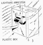
arrestor in a plastic box with a tight-fitting lid. Cut holes in the side of the box to accept the lead-in wire; drill holes in the bottom to fit the arrestor's mounting screws.—JOHN A. COMSTOCK.
