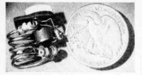
Photo compares transmitter with 50¢ piece. It consists of one variable and two fixed ceramic capacitors, tuning coil and the diode itself—inside can in center of transmitter.
