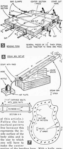
portion of the bending form. With a knife, carefully cut out the drawing. Draw in the neck and tail blocks, but do not cut them out at this time.
