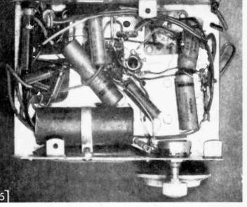
Underside of a four-tube set with hand-wired components and conventional metal chassis. Its circuit is identical to that of the printed set, but note the "jungle" of parts.
