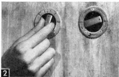
2 Balance controls on side of cabinet permits adjustment of speaker to room in which it is placed.
