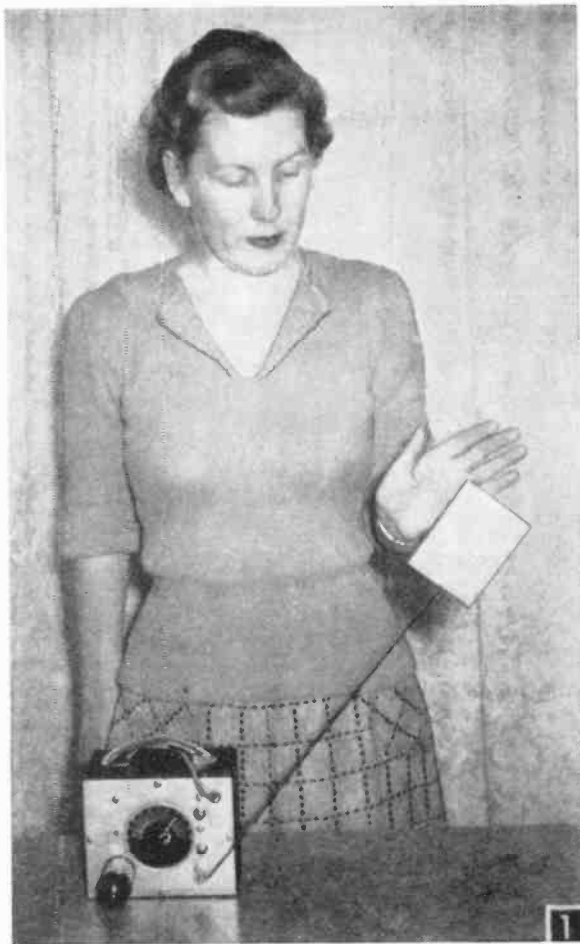
Hand approaching metal plate causes the lamp plugged into control receptacle to light up. Bells, motors, etc. may be plugged into the 110-120 v outlet.
