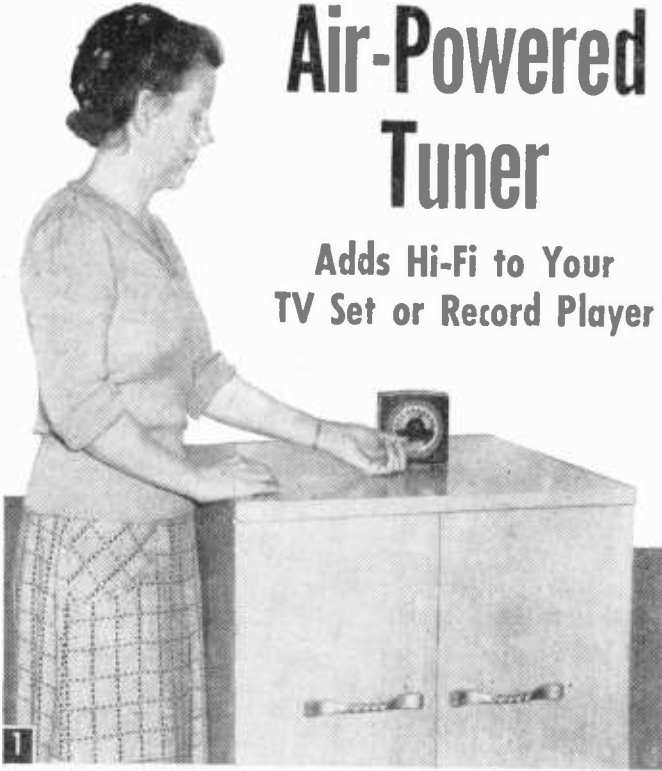
This little tuner brings hi-fi radio reception to TV when plugged into the set's "phono jack." Photo above shows how an old alarm clock case provided a neat cabinet for the tuner.
