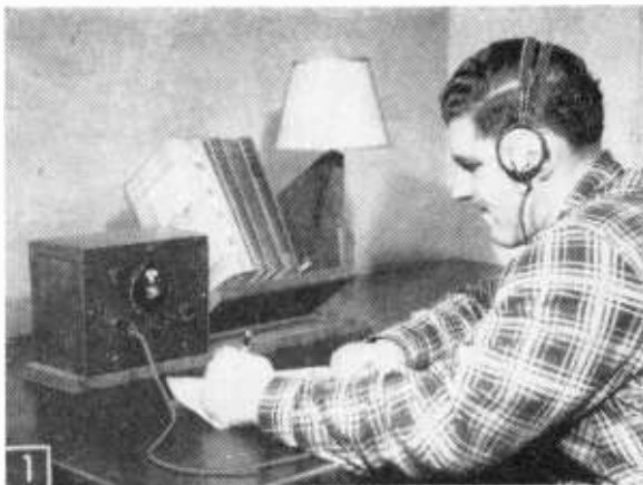
Designed primarily for use by the student ham who wants to keep up his code speed, the Student's Special can be modified to receive the standard broadcast band.
