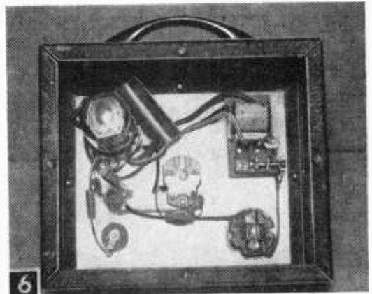
Looking into rear of control box with cover removed. Front panel and chassis are one, making for simplified construction.
