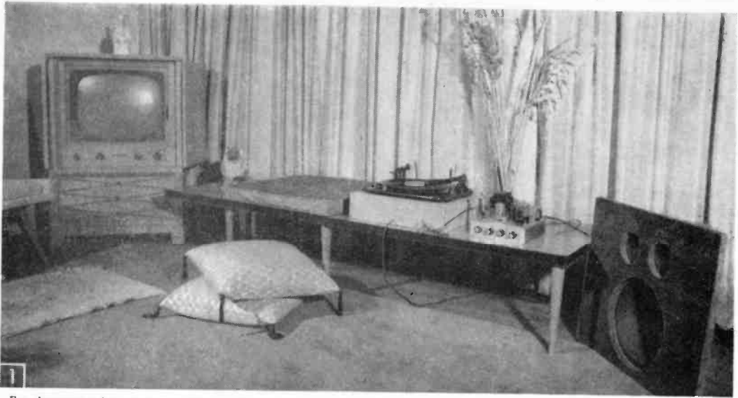
For demonstration purposes, this is all you need for stereophonic sound. Here a record changer with stereo pickup (center) simultaneously feeds the small amplifier on bench next to it and in turn the temporary speaker assembly at right from one channel of the stereo disc, and feeds the amplifier and speaker unit in the TV set at left from the other channel. Distances are about right for stereo listening in the average living room.
