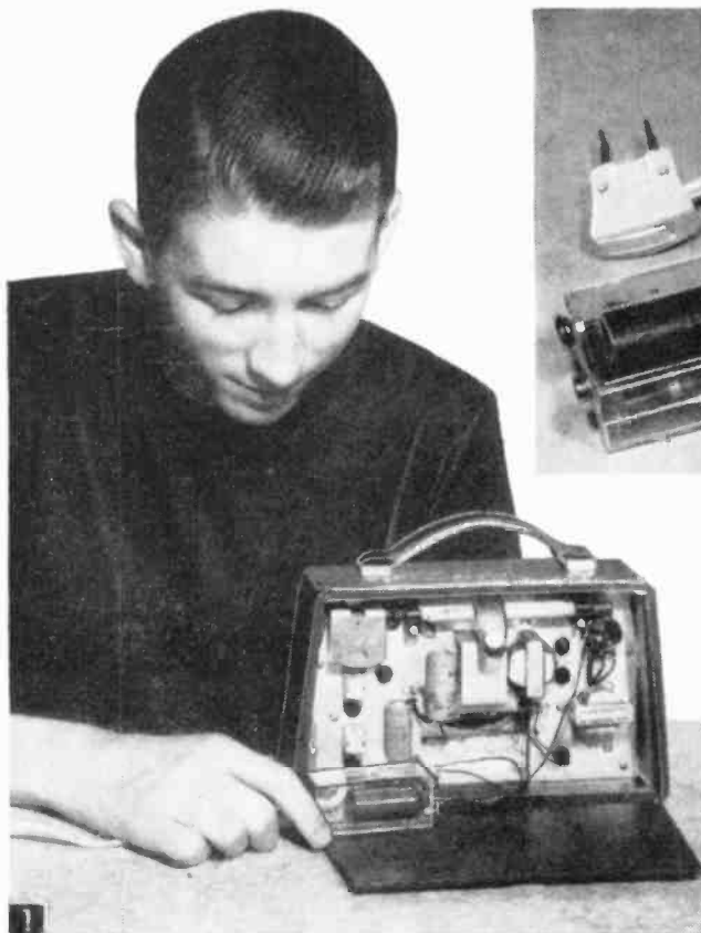
Battery eliminator (above) built into hinged plastic box delivers 9-volts to this six-transistor set.
