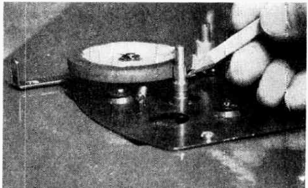
Fig. 3. The 78 rpm aluminum collar has been removed by loosening spline set-screw. Pencil points to part of motor shaft that has been filed down to .263 in. or just enough to give exactly 45 rpm. Aluminum collar can be put back for 78 rpm.
