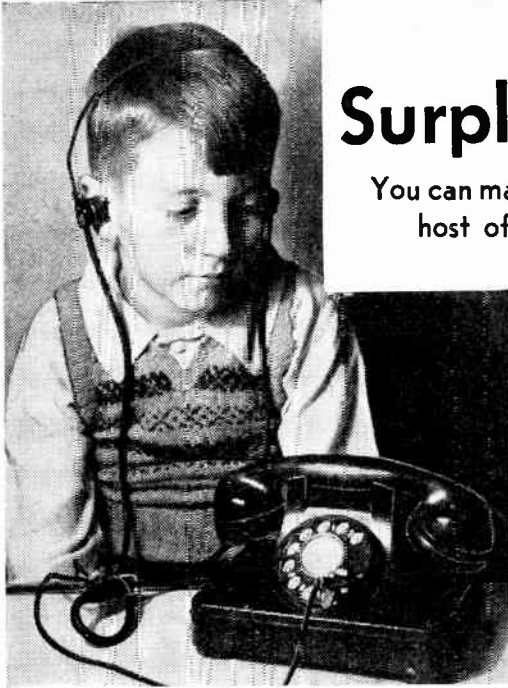
Nothing to tune, nothing to get out of order with peppy little set "built-into" surplus headset. Telephone dial stop provides clip-on antenna. Phone shown came from French liner "Normandie."
