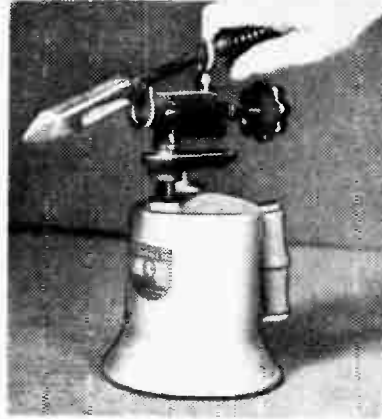
Fig. 3. Heating a conventional soldering iron with a blowtorch.
