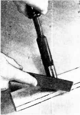
Fig. 13. Support the electric iron on a block of wood when cleaning the point.
