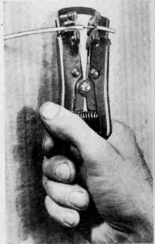
Fig. 20. An insulation stripping tool.
