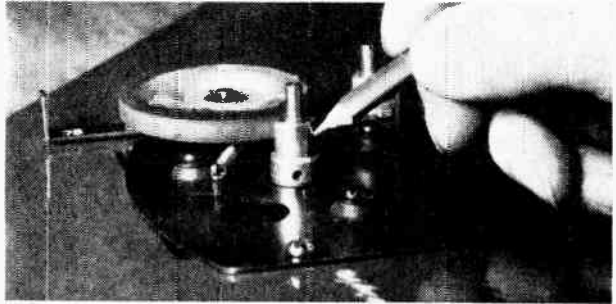
Fig. 2. The works of the General Industries Model-DR dual-speed phono motor. Pencil points to the 78 rpm diameter on removable aluminum collar over motor shaft.
