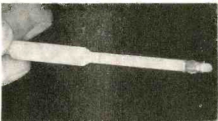
Fig. 4—A programming clip ready to be inserted into a channel hole.
