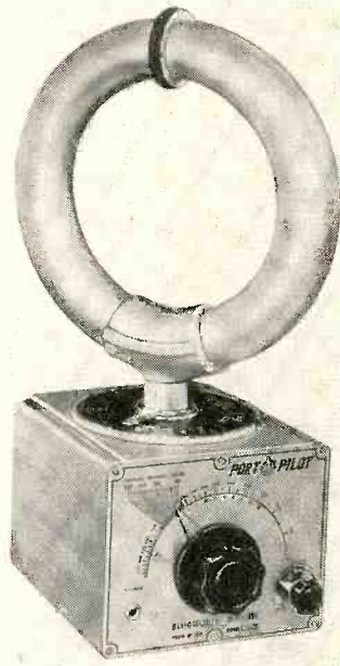
Photo of a typical direction finder using a loop antenna.
