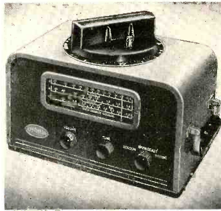
A three band direction finder employing a ferrite loop.
