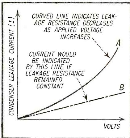
Fig. 3—The variation of leakage resistance with applied voltage is shown in the above illustration.
