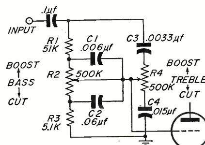
▶ Fig. 3—Universal Losser circuit used in G.E. A1-200 preamplifier.
