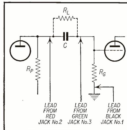
Fig. 7—Coupling capacitor leakage check with "three-lead" test.
