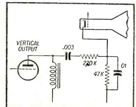
Fig. 6—Vertical blanking pulse being fed to cathode of the CRT.
