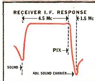
The adjacent sound carrier has been suppressed by some 50 db, which: (1) Enables the signal level of the desired channel to control the AGC action of the receiver. (2) Completely removes the "beat", leaving a clear, strong picture.
