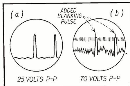
Fig. 8—Two views of the blanking pulse on the oscilloscope screen.
