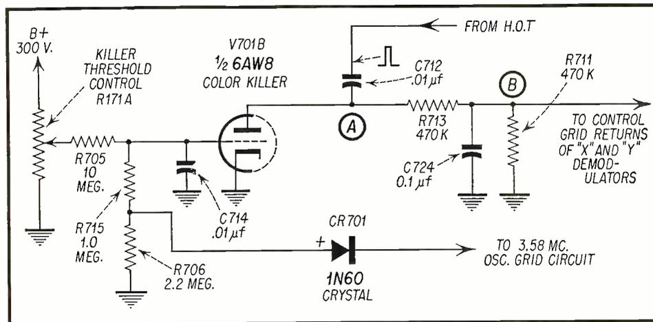
Fig. 3—Color killer circuit of the RCA CTC5N bias obtained from burst-APC chain.
