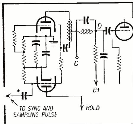
Fig. 9—Typical synchroguide circuit. B+ applied at point C caused the trouble in this case.
