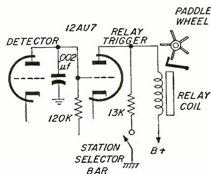
Fig. 2—Partial schematic of the Delco "Signal Seeking" auto radio with detector and trigger circuit.
