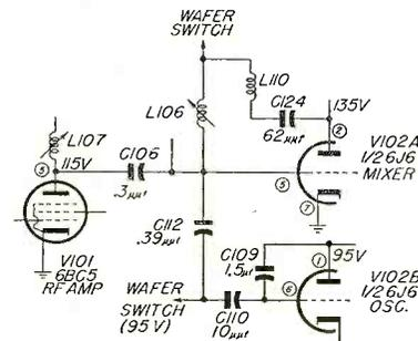
Fig. 1—Partial schematic of tuner circuit of GE "F" series chassis.
