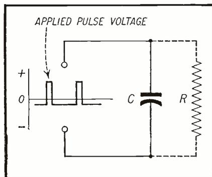
Fig. 6—If the condenser is good, action is same as with resistor.
