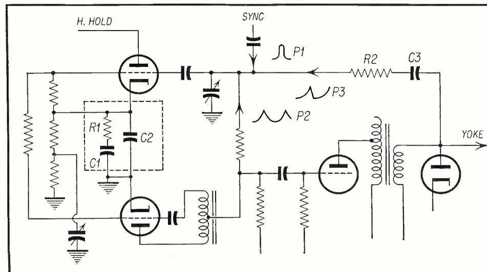
Fig. 2—Typical pulse width *afc* circuit. The component wave-forms used to produce the automatic control action are shown as P1, P2, and P3.
