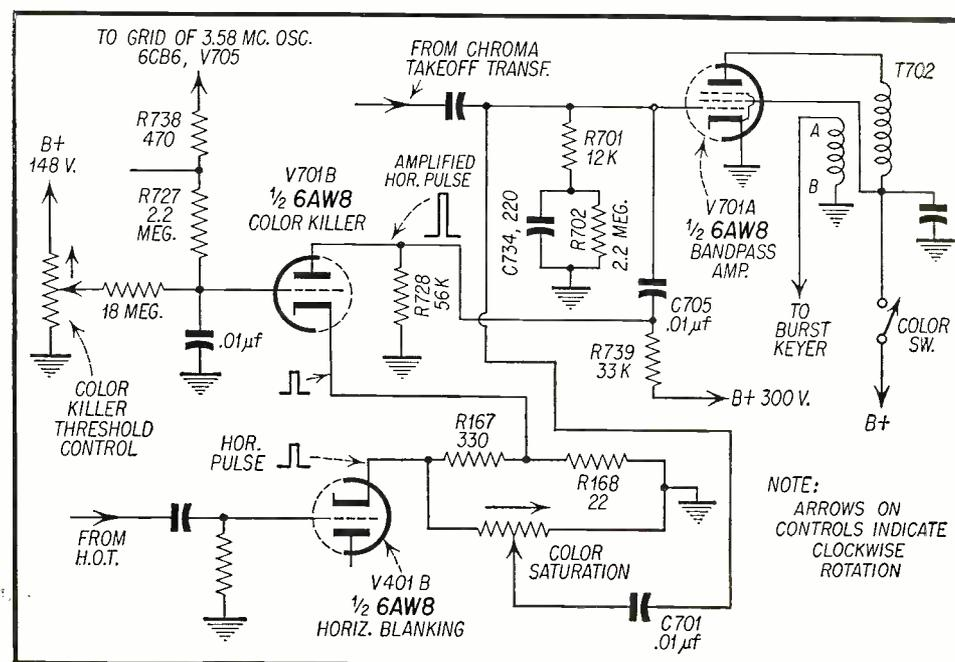
Fig. 2—Color killer circuit of the RCA CT5. Note the use of an auxiliary switch.
