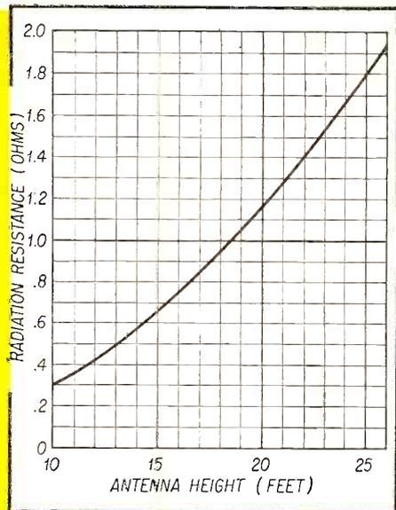
Fig. 1—The radiation resistance of Marconi antennas having heights that vary from 10 to 26 feet.
