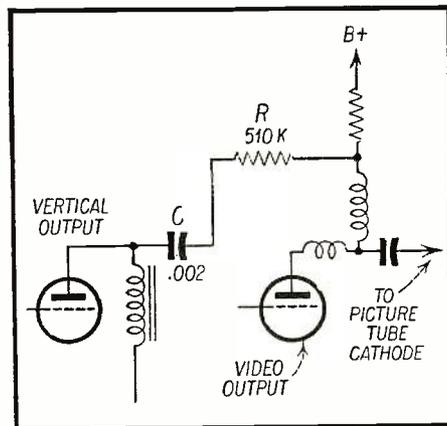
Fig. 7—Blanking pulse injected into video amplifier plate load.
