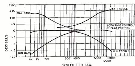
Fig. 6—Typical compensation curves showing range of control with universal loss.
