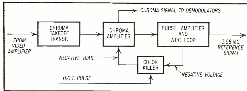
Fig. 1—Block diagram to illustrate the action in a typical color killer circuit.
