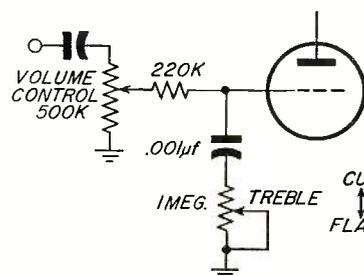
▶ Fig. 2—A simple, basic, treble-cut tone control circuit.
