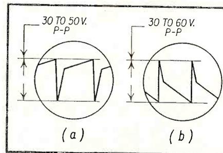
Fig. 5a—Negligible slope in the portion following the pulse.
