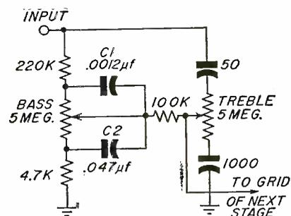
Fig. 5—Tone control circuit of the Pilot PA-913 control unit.
