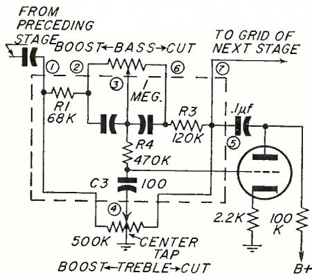
Fig. 7—Feedback tone control featuring variable cross-over.
