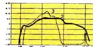
3 This is the frequency response curve of a conventional P. A. horn.
