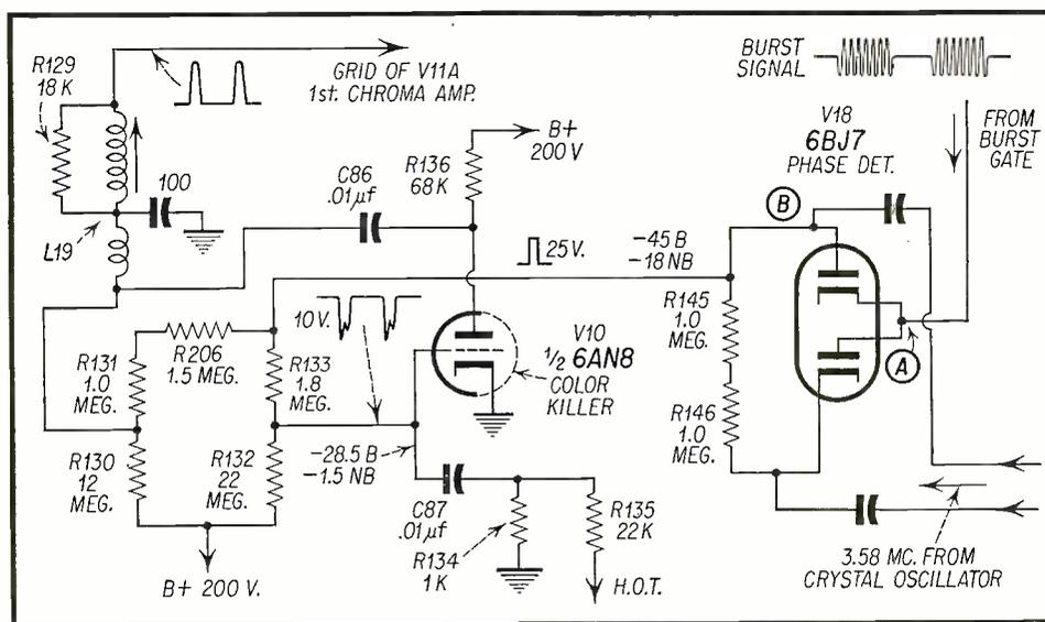
Fig. 4—Partial schematic showing color killer circuitry of the Emerson 120319-D.
