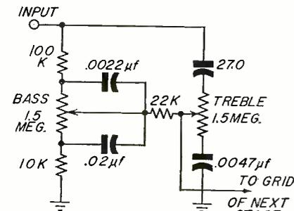
▶ Fig. 4—Universal Losser circuit. Harmon-Kardon C-100 amplifier.
