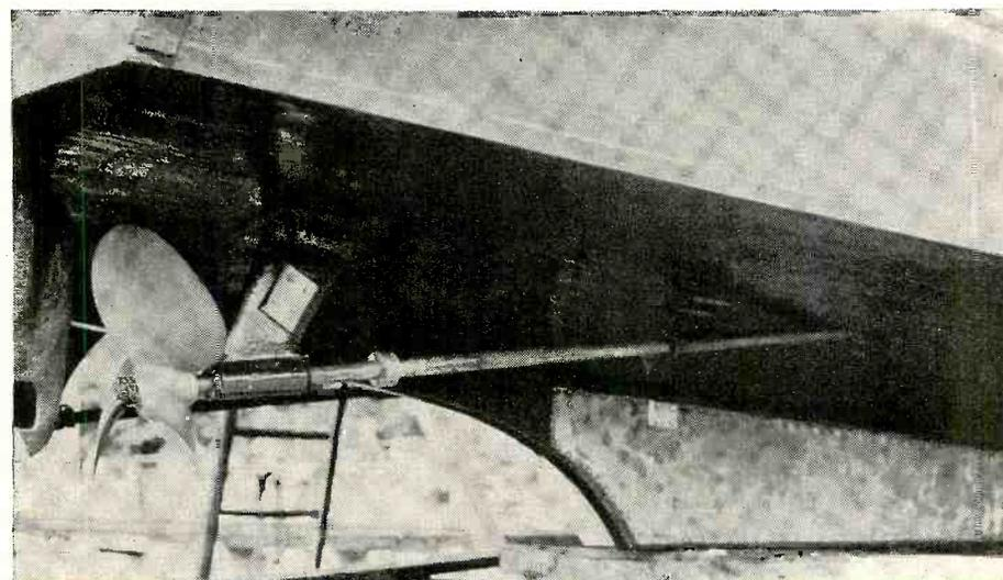
Practical method of installing ground plate on deadwood.
