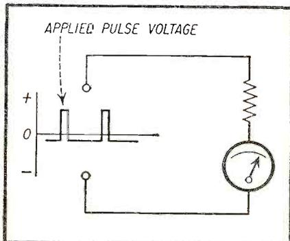
Fig. 5—The average current flow in resistor due to pulse is zero.
