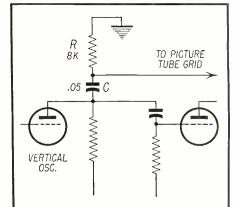
Fig. 3—A simple circuit which is commonly used to obtain vertical retrace blanking. The  $.05 \mu\text{f}$  condenser and the 8K resistor are the added components.
