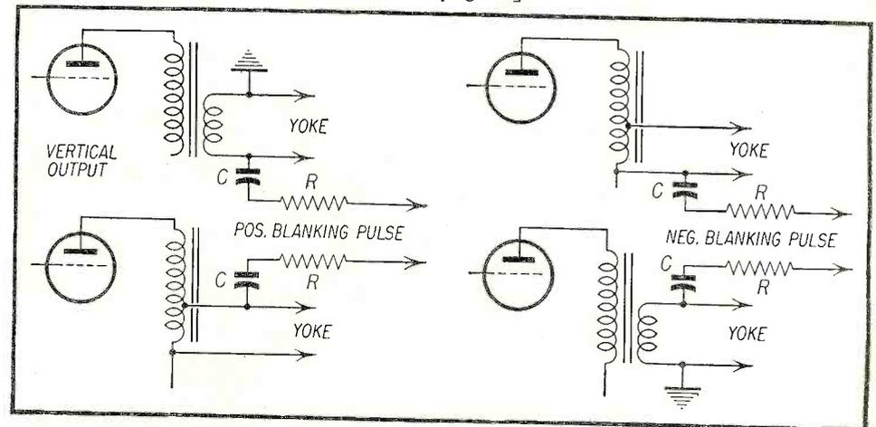
Fig. 4—Four commonly used circuits for supplying vertical retrace blanking. Note that two of these supply a positive blanking pulse and two a negative.
