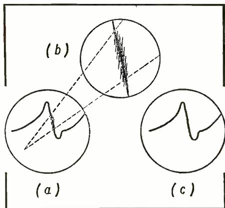
Fig. 1a—Distorted wave form at plate of sync amp; Fig. 1b shows an expanded view of the distortion. Fig. 1c shows the appearance of the normal wave form.
