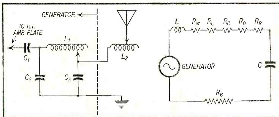
Fig. 2—The practical transmitting and equivalent circuits.
