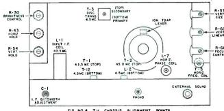
FIG. NO. 4 T.V. CHASSIS ALIGNMENT POINTS
