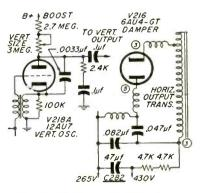
Fig. 1—DuMont RA-340 chassis B plus boost and vertical circuit.
