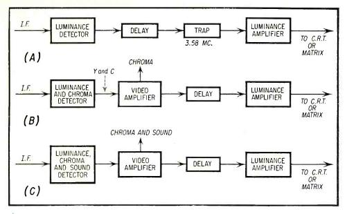
Fig. 1—Three types of luminance systems found in color TV receivers are shown in block diagram form with chroma and sound take off points.
