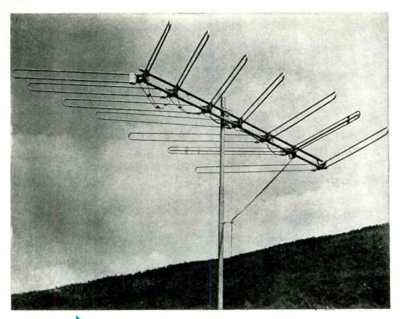
Fig. 1—Seven element terminated travelling wave antenna.
