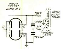
Fig. 3—Partial schematic showing Crosley 477 chassis afc circuit.
