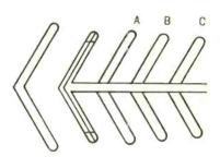
Fig. 8-Position of dipoles. Impedances decrease from feed point to shortest dipole.
