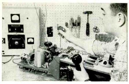
Fig. 1—Compromise measures such as coil-clip tuning are still used, as seen in this photograph, for reasons of economy.
