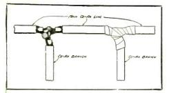
Fig. 1—Original method of tapping transmission lines.
