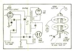
Fig. 2—Horizontal deflection circuit of RCA KCS48T chassis.
