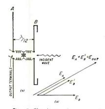
Fig. 5—The basic elements and a vector relationship for low band operation without signal delay.
