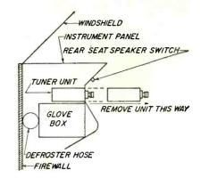
Fig. 5-Tuner unit is removed by bringing it forward and out.
