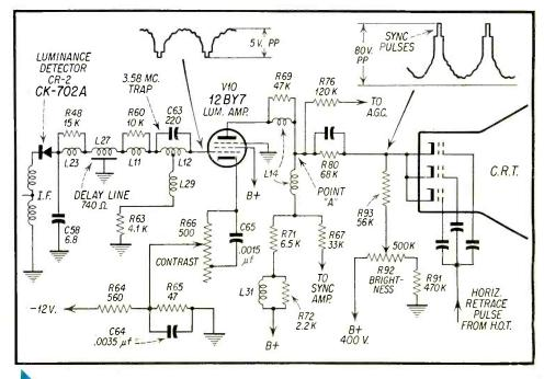
Fig. 2—Partial schematic of luminance section of Sentinel Model 1U-816.
