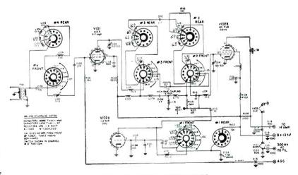
Fig. 2. Schematic Diagram VHF TUNER RJX-064
