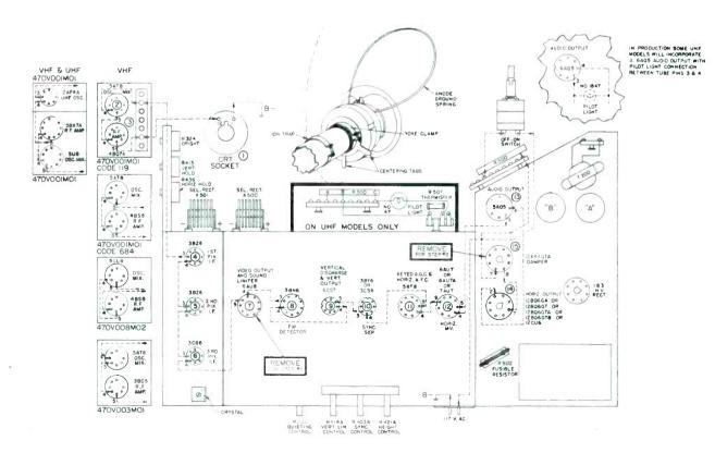
Top View of Sockets for Heater Check
