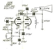
Fig. 2—Vertical output and blanking circuit of G.E. "N" chassis.
