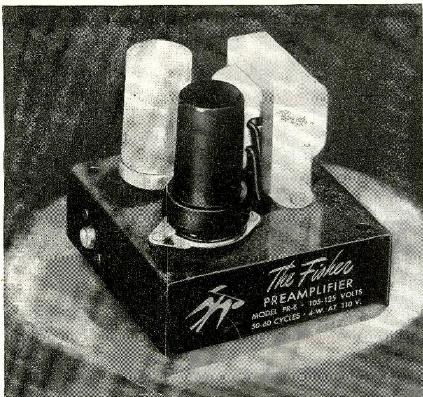
Fig. 4—Above is shown a picture of the Fisher Model PR-6, a self-powered preamplifier which employs fixed equalization.
