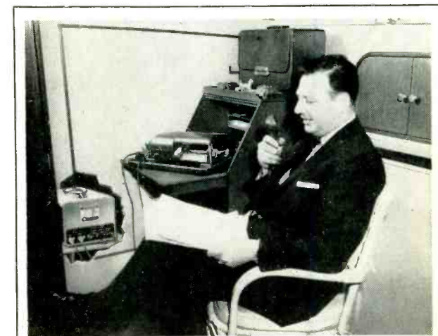
Cornell-Dubilier Powercon converter supplying 110 V.A.C. household power from boat battery system to dictation machine.
