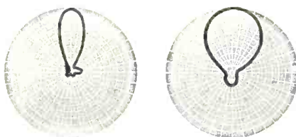
Fig. 16—Directional patterns of the Amphenol Poweray antenna.
