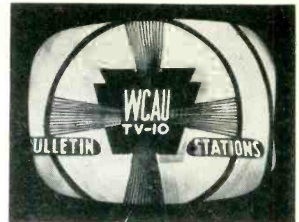
Fig. 7—This figure illustrates low sync amplitude.
