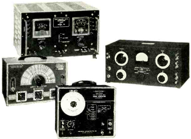
Various commercial sine and square wave generators. Top left is the Hickok Model 710; middle left is the EICO Model 377; middle right is the Measurements Corp. Model 71; and bottom is the Precision Series E-300.
