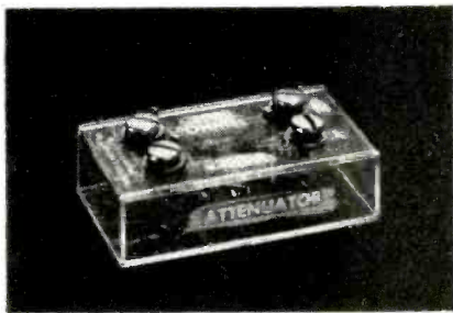
One of the 300/300 ohm, 20 db attenuators listed in Table 1 assembled in small plastic container.
