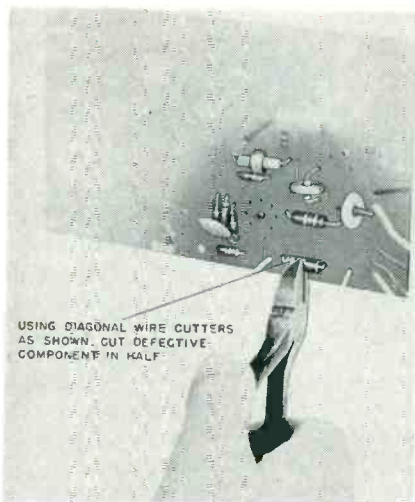
Fig. 2—Cutting a defective resistor apart so as to have maximum lead length left.
