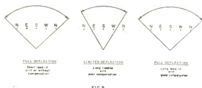
Fig. 5—Full deflection of control unit needle is shown—when a rotator's long lead-in is compensated. Note contrast with full deflection and limited deflection.
