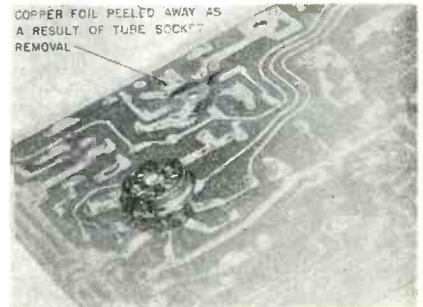
Fig. 10—The manner in which the metal grounding foil breaks away because of tube socket removal.
