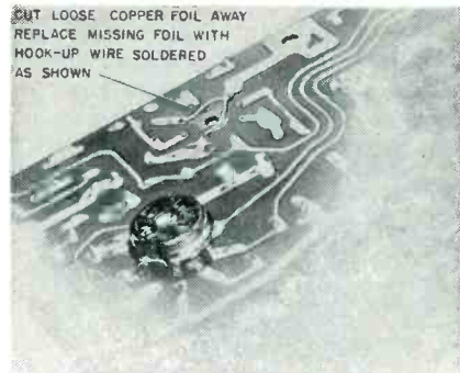
Fig. 11—A jumper wire may be used to replace the missing metal foil, as illustrated here.
