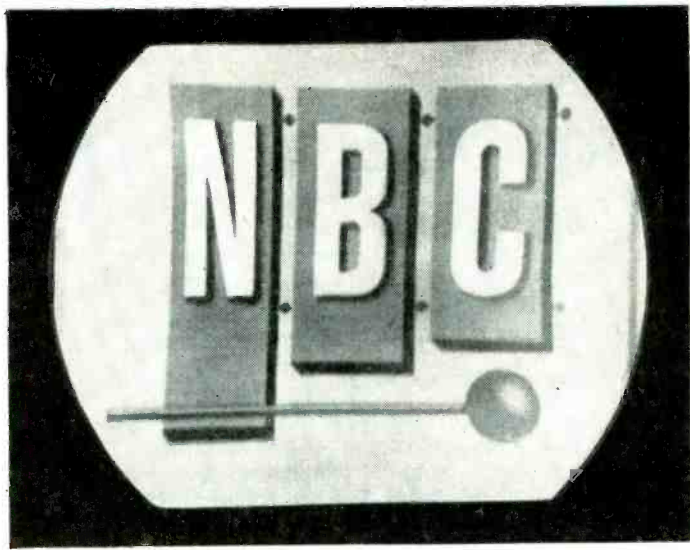
Fig. 2—Color stripe appears as light green bar. On black and white sets bar is almost invisible.
