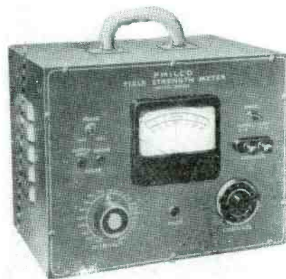
Fig. 1 —Physical appearance of the Philco Field Strength Meter, Model M8104. Note sturdy construction and accessibility of controls.
