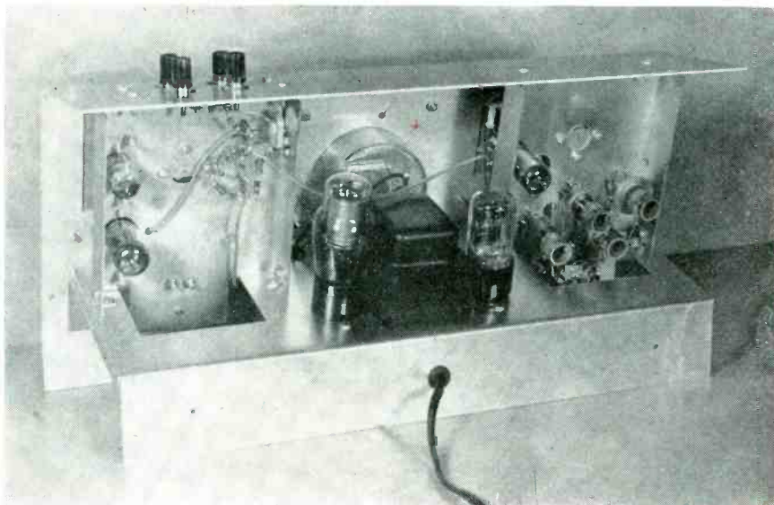
Fig. 5—Inside view of completely assembled Q-Meter. The vertically mounted Q subchassis is seen on the left. The generator subchassis is mounted vertically on the right. Power supply components and Q voltmeter are seen in the center. The complete instrument is 16\frac{1}{2} \times 8 \times 5\frac{3}{4} .
