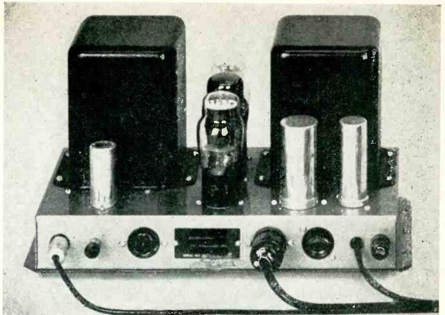
Fig. 5—Trend in modern wide range amplifiers is shown in the size of the power and output transformers, which dwarf the 6L6 tubes above. This amplifier is conservatively rated at 20 watts. It employs only one 12AX7 and the output stage.
