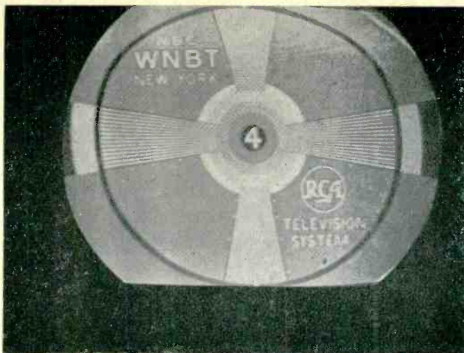
Fig. 4—Pattern produced when 4.5 mc reaches the grid of the picture tube.
