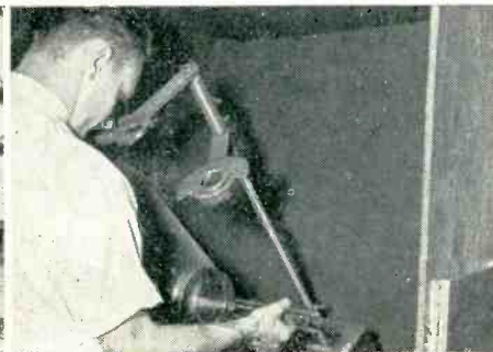
Examination with polarimeter permits careful control of strains for superior glass-to-metal sealing.
