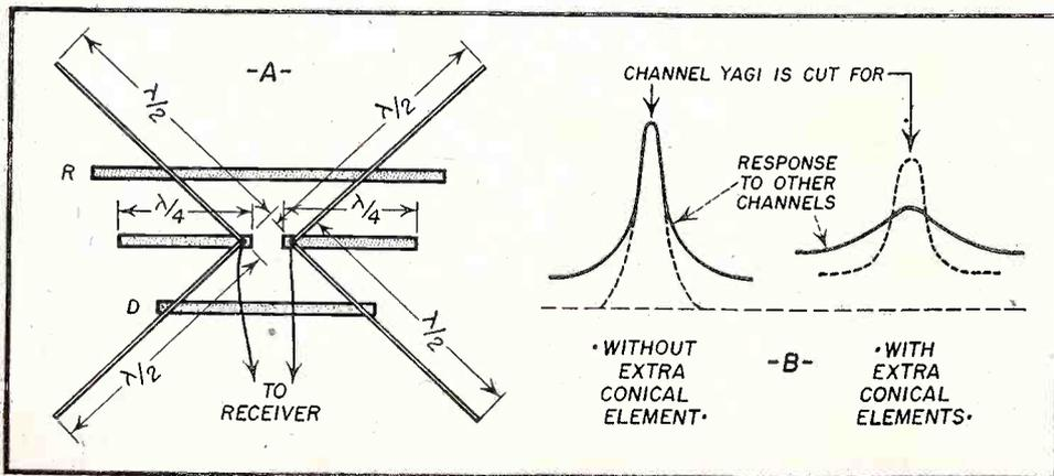
Fig. 8. Adding extra conical elements to an array for broadband response with a peak on one channel.
