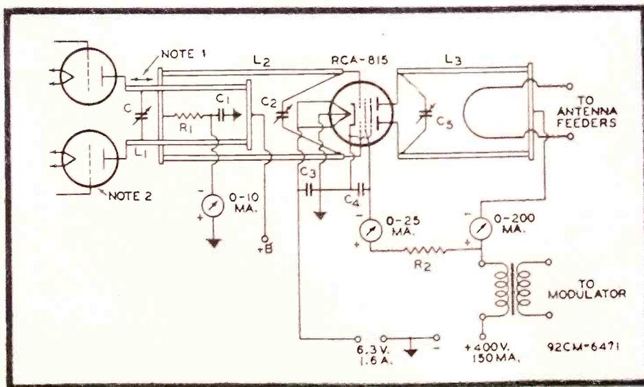
Fig. 4. Recommended circuit for 815 tube when being used in vicinity of 100 mc.
