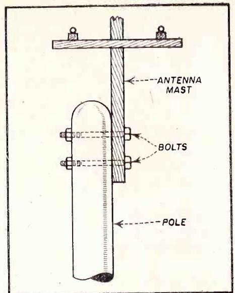
Fig. 5. Mounting an antenna mast on a pole.
