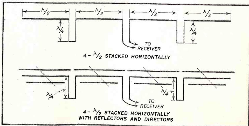
Fig. 2. Examples of horizontal stacking with driven elements and with reflectors and directors.
