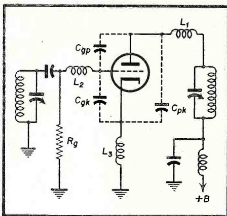
Fig. 1. Tuned plate-tuned grid oscillator with conventional circuit elements.
