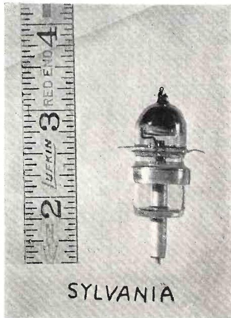
Fig. 8. Sylvania rocket tube 2C37.
