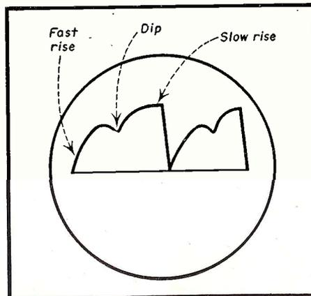
Fig. 7. Deformation of sawtooth waveform sweep for defect shown in Fig. 5.
