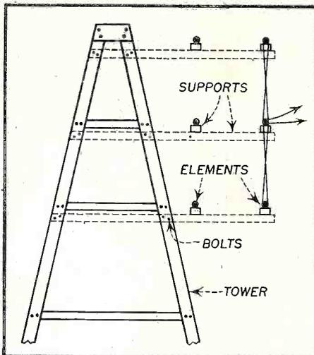
Fig. 6. Mounting arrays on side of a large tower.
