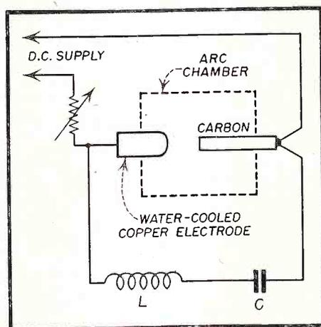
Fig. 2. Poulsen arc converter
