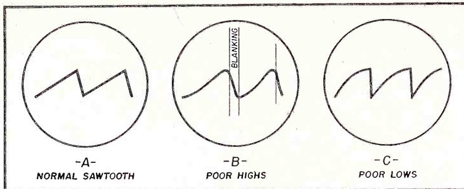
Fig. 9. Effects of poor frequency response circuits on sawtooth linearity.
