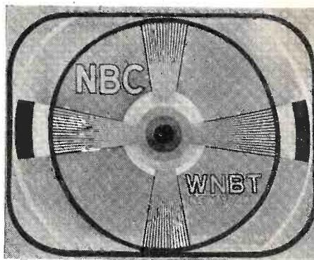
Fig. 4. Test pattern with good linearity.
