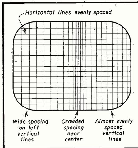
Fig. 6. Type of cross-hatch pattern produced by linearity pattern generator for defects shown in Figures 5 and 7.
