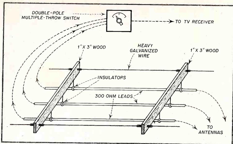
Fig. 7. Carrying multiple leads into receiver.
