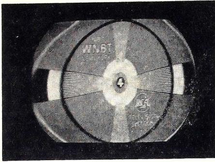
Fig. 5. Defects due to non-linearity of horizontal sweep sawtooth.
