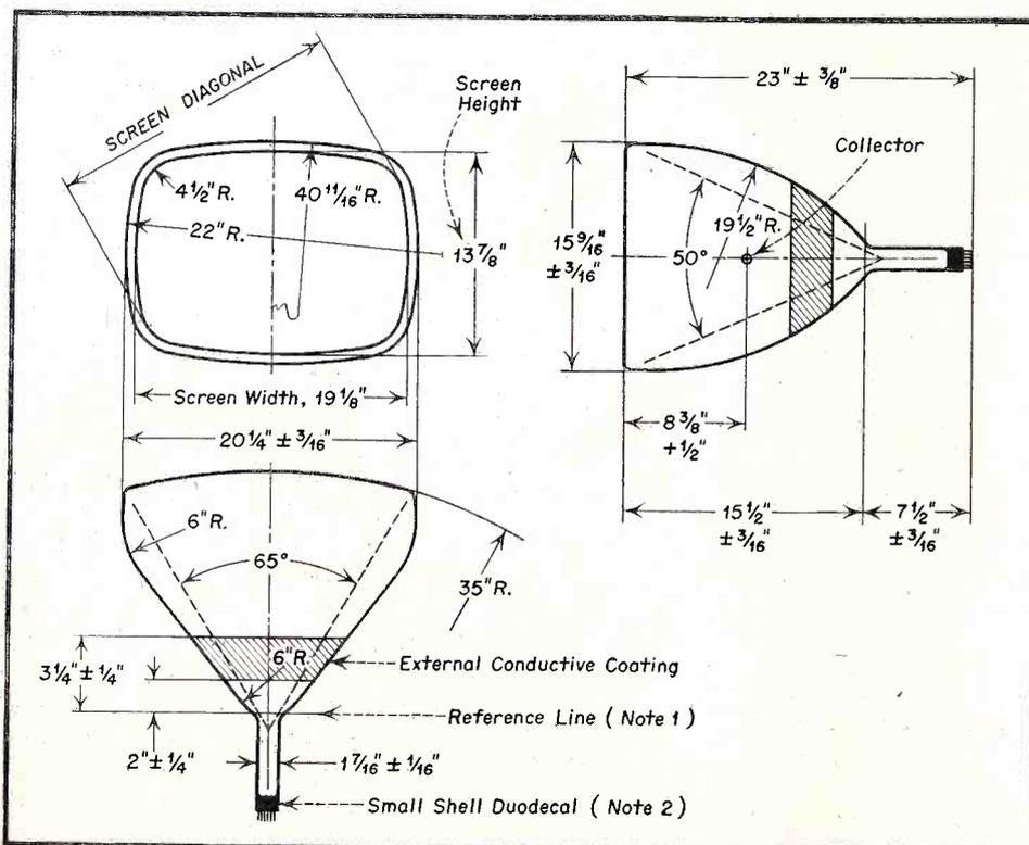
Fig. 1. New type cylindrical-face picture tube designed to eliminate reflections.
