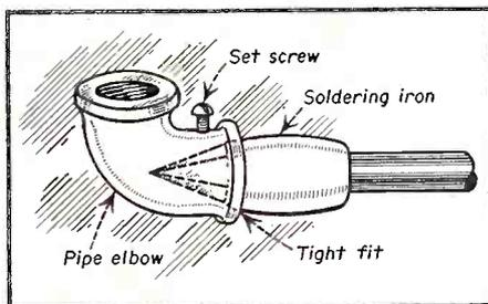
Fig. 2. Solder pot made from pipe elbow which can be used for tinning wire ends.
