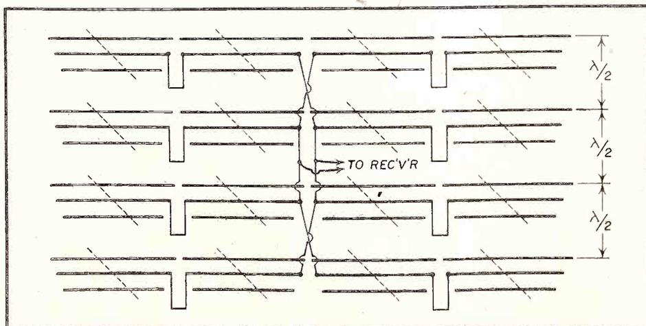
Fig. 3. Example of array combining horizontal and vertical stacking.
