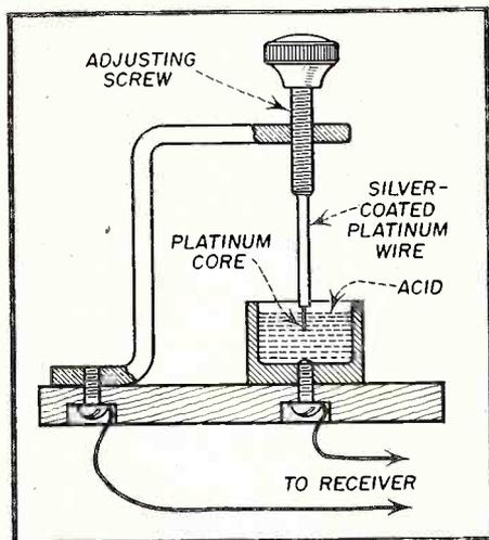
Fig. 1. Electrolytic detector
