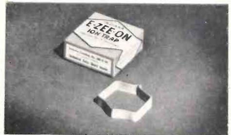
on, grip-slug beam bender made of one piece, permanently magnetized Cunife that can't be put on backward and requires no manual clamping. According to the manufacturer, the "E-Zee-On" provides a more uniform magnetic field pattern, resulting in brighter, more uniform definition easily attained by sliding the "E-Zee-On" forward or backward on the tube neck. Because of its uniform weight distribution, it will not jar loose or slip, nor come out of adjustment.
