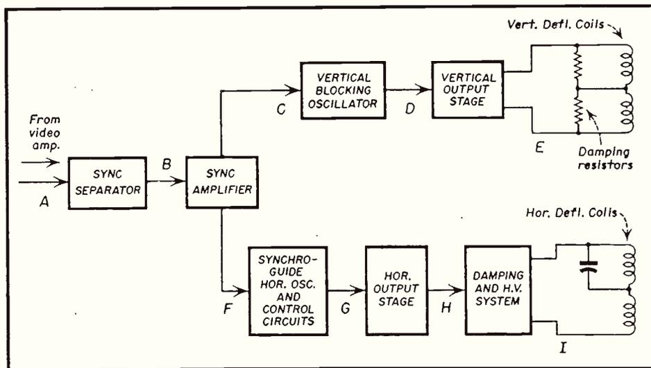
Fig. 1. Identification points for checking typical television receiver.
