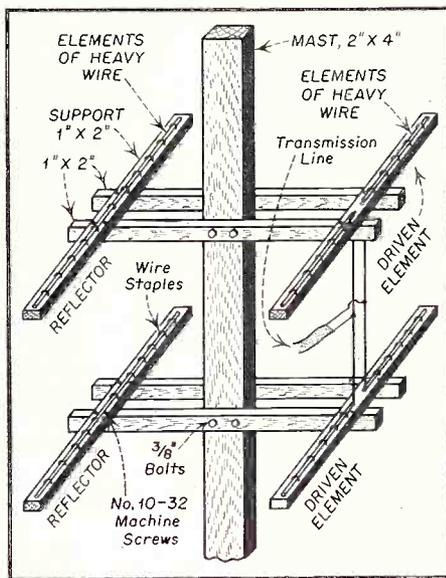
Fig. 4. Antenna construction using wooden framework.
