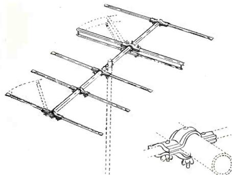
Examination of the RMS construction discloses rib re-enforcement, with double brackets to provide sturdy, stress-proof performance. Both sides of each element are locked in the clamp support, in three positions.
