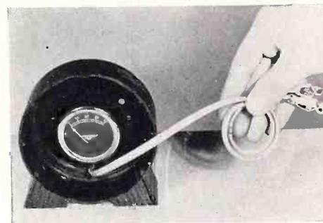
Fig. 3. Utilizing old clock case as meter mount.
