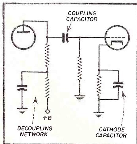
Fig. 11. Circuit capacitors which are likely causes of poor low frequency response.
