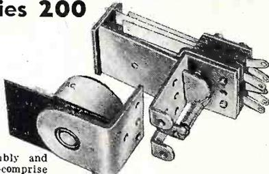
Two basic parts—a coil assembly and a contact switch assembly—comprise this simple, yet versatile relay. The coil assembly consists of the coil and field piece. The contact assembly consists of switch blades, armature, return spring and mounting bracket. The new Guardian Midget Contact Assembly which is interchangeable with the Standard Series 200 coil assembly, is also available in either single pole, double throw; or double pole, double throw.
