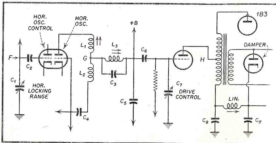
Fig. 3. Location of test points in Synchroguide horizontal system.
