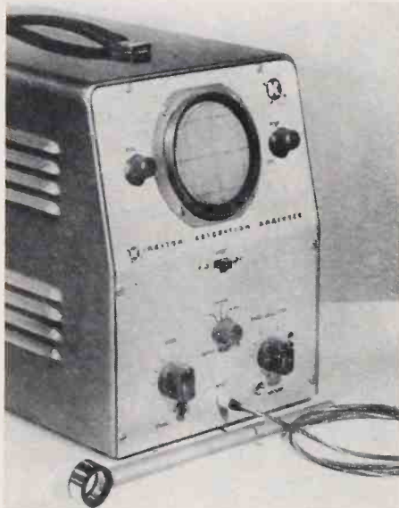
Fig. 1—Absorption analyzer and probe. Note the few controls.
