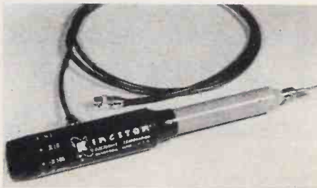
Fig. 3—This probe permits the analyzer to be used as a scope.
