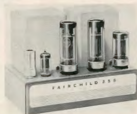
Fig. 1—Fairchild Model 255A 30 watt power amplifier.
