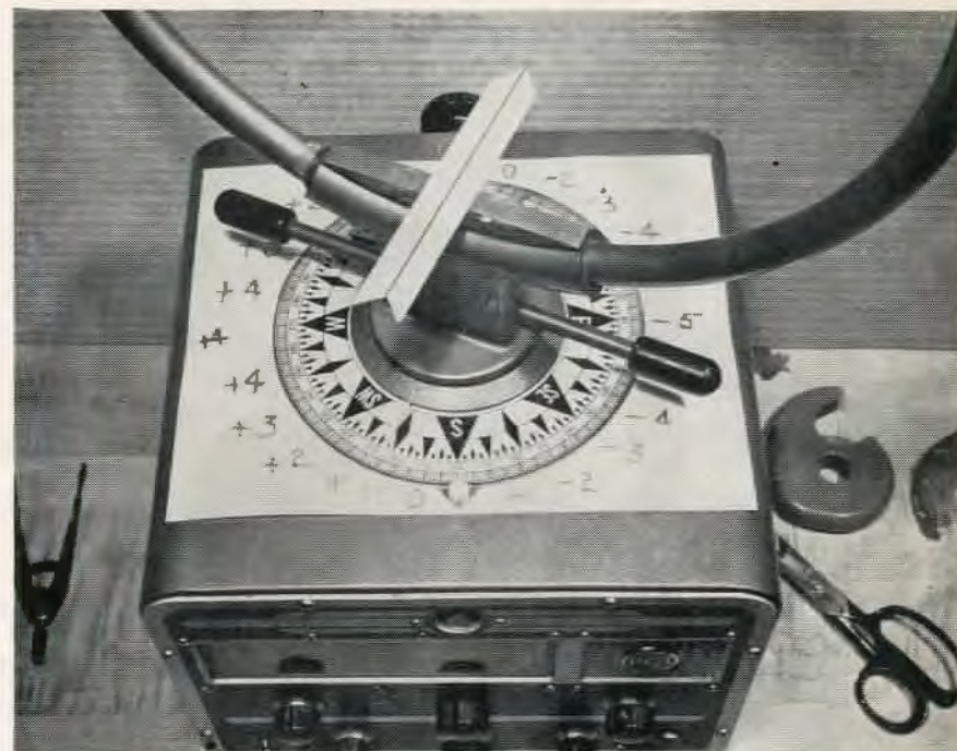
Fig. 1—A cardboard arrow pasted along the null line for visual bearings.
