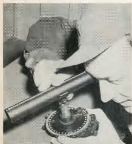
Fig. 2—Accurate visual bearings may be made with a pelorus.
