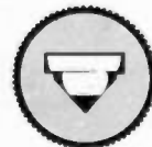
Shaft position in knob requiring 3/32" flat.
