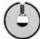
How shaft is positioned for set-screw knob.
