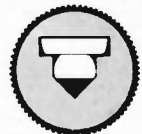
Shaft position in knob requiring 1/32" flat.
