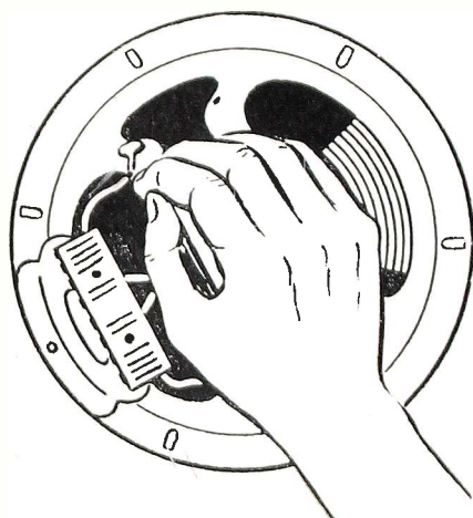
Fig. 6—Cement paper ring and place in position, making sure mounting holes are lined up. Turn speaker on face and allow to dry thoroughly, at least 2 hours.
