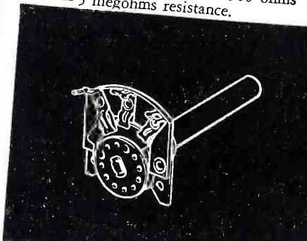
AUXILIARY SPEAKER SWITCH: Three position switch to provide remote control for auxiliary speaker installations. Life test — 10,000 cycles. Rating 6 watts.
