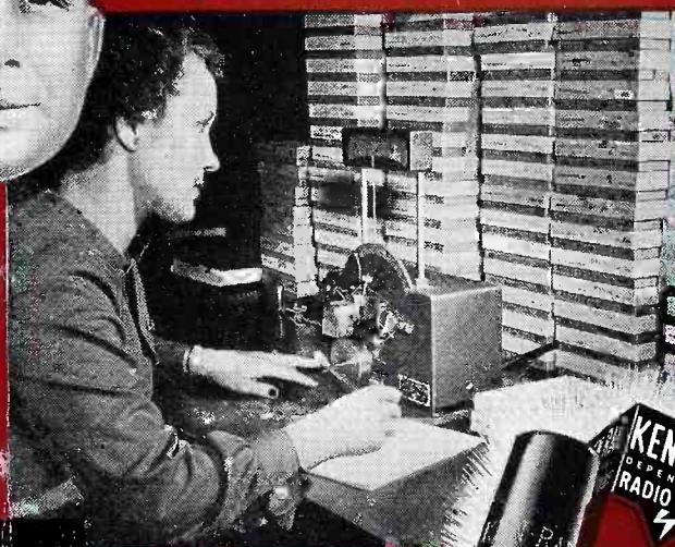
WALTER DOWNING , Foreman, Raw Materials Inspection Department, is in charge of comprehensive testing of all materials used in making Ken-Rad tubes. Here cathode sleeves are being tested for breaking strength.
