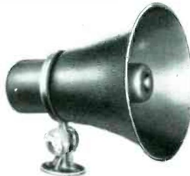
**NEW SMALL RE-ENTRANT HORNS**, extremely efficient for factory inter-com and paging systems; for sound trucks, R.R. yards and all other industrial installations where high noise levels are prevalent. Watertight, corrosion-proof, easily installed. Two new models — type RE-1 1/2, complete with Baby Unit, handles 25 watts, response 300-6000 cps. type RE-12, complete with Dwarf Unit, handles 10 watts, freq. response of 400-8000 cps.
