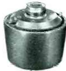
**NEW SPECIAL PM HORN UNIT**, having Alnico V magnet ring, completely watertight, encased in a heavy aluminum spinning. Provides extremely high efficiency reproduction with minimum input. Handling capacity 35 watts continuous, 60 w peak.
