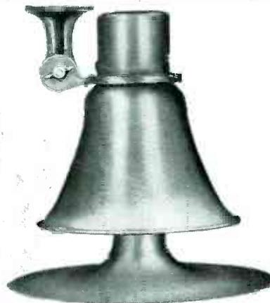
**NEW RADIAL RE-ENTRANT SPEAKER**, excellent for all types of industrial sound installations. Provides superlative and complete 360° speech intelligibility by efficiently over-riding factory high noise levels. Frequency response 300-6000 cps. Handling capacity 25 watts continuous, 35 w. peak. Has mounting bracket. Size 12" wide by 12 1/2" high.
