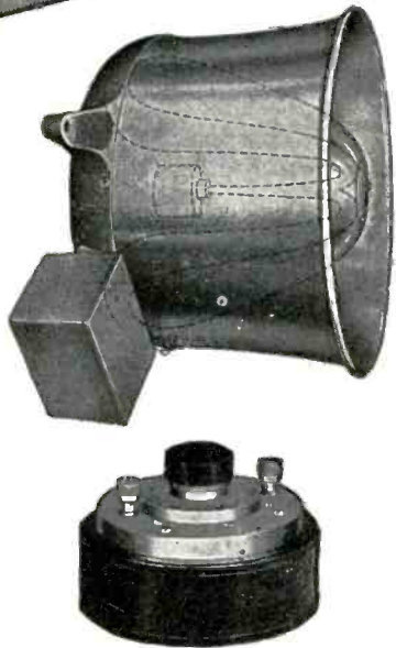
The RACON Marine Horn Speaker is used both as a loudspeaker and as a microphone. Approved by the U. S. Coast Guard for all emergency loudspeaker systems on ships. A double re-entrant type speaker, completely waterproofed and weatherproof. Ideal for general P.A. and Marine use. Several sizes available. RACON Permanent Magnet Horn Units are available in operating capacities of from 10 to 50 watts.
