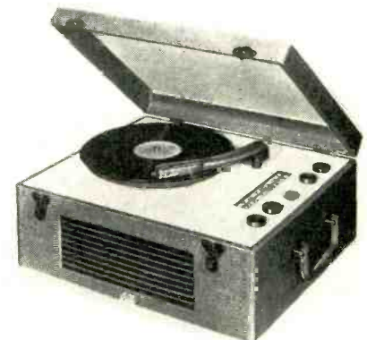
ECA , model 105, 5-tube portable radio-phonograph. Two-tone leatherette cover with carrying handle. 1-watt output. 5" alnico V speaker. Tuning range 540-1700 KC. Slide rule illuminated dial. Di-fusa-tone grill. Built-in loop antenna; tone control; light weight crystal pickup. Electric Corp. of America, 45 W. 18th St., New York 11, N. Y.
