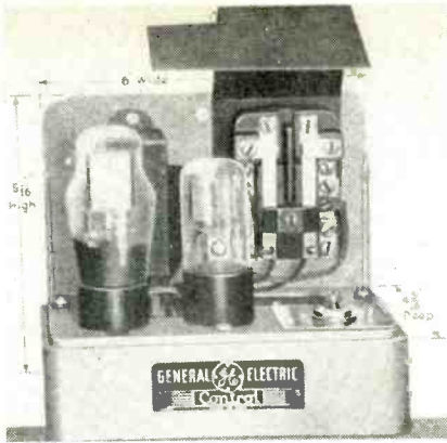
Fig. 7—A G.E. photoelectric control general purpose relay using a phototube and thyatron. Note compactness of unit from the dimensions shown.
