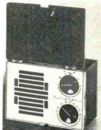
MOTOROLA , model 5A1 "Playboy" battery portable. Uses miniature "Handie Talkie" type tubes. PM speaker. Loop antenna mounted in front cover. Tuning range 550-1600 KC. Automatic switch turns set on when cover is opened. Model 5A5, operates ac-dc and battery. Galvin Mfg. Corp., 4545 W. Augusta Blvd., Chicago, Ill.
