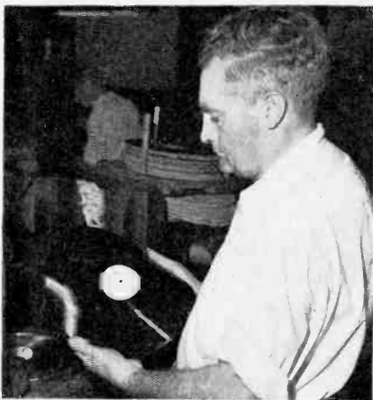
NON-BREAKABLE RECORD: First non-breakable, high fidelity plastic phonograph record for home use is taken off the press by Arch Sterling, at RCA Victor plant in Camden, N. J. Developed after 11 years of research, it can be played on all home phonographs. First of these discs will be released in October.
