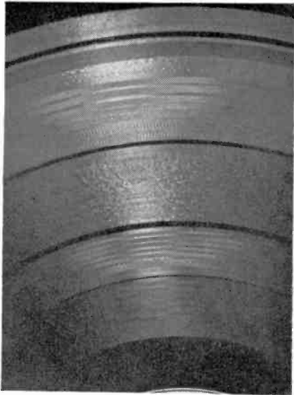
Well-spaced grooves except where they are cut too deeply, as in darker band in second group where spiral shadow appears. Shadow would show as series of coarse spirals if continued across entire record. This is indication of turntable rumble that reproduces as a low-pitched hum.
