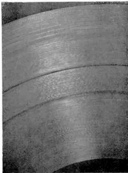
Appearance of "twinning". Instead of being evenly spaced, the grooves occur in pairs with little wall between them. Grooves are apt to cut over at first playback, causing a "repeat".
