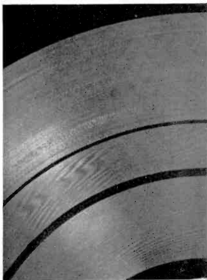
Outside band: Modulated grooves of music recording. Center band: Pattern created by excessive 120-cycle amplifier hum. Inside band: Pattern caused by 60-cycle hum in amplifier.
