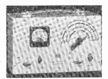
The VSM2, one of a range of signal strength meters manufactured by J. S. Fielden. It is continuously tuneable over Bands I, II and III.
