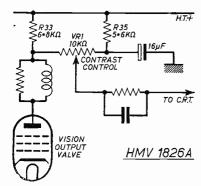
contrast control in a rather complex arrangement around the video amplifier stage. The anode voltage for this valve was checked and thought to be somewhat low, but this was dismissed as of little consequence.
