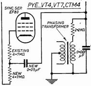
A positive cure for this is to change the grid resistor to the sync separator for two  $4.7 M\Omega$  resistors in series, instead of one single  $4.7 M\Omega$  resistor. The junction of the two resistors is taken via an additional  $0.05 \mu F$  capacitor to the junction of the  $0.001 \mu F$  capacitor and  $2.2 M\Omega$  resistor which are across the phasing transformer. All other components remain as before.
