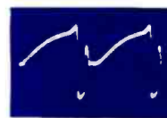
17 CR501 Cathode 12V P-P Horiz. Rate Horiz. Phase Detector
