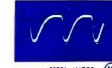
SR201 ANODE HORIZONTAL PHASE DETECTOR HORIZONTAL RATE 15V P-P
