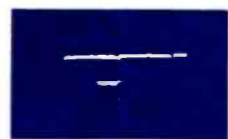
V105 PIN 2 KINESCOPE GRID VERTICAL RATE 80V P-P
