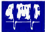
2 2 VOLTS P/P, 15,750 HZ (MAX. CONTRAST)
