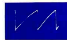
V206A PIN 2 VERTICAL OUTPUT GRID VERTICAL RATE 28V P-P
