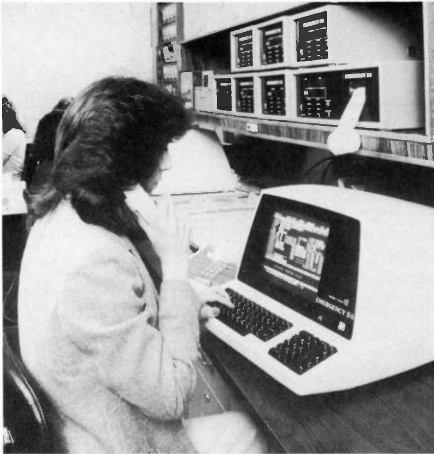
Figure 10: Computerization speeds the processing of alarm signals through the monitoring facility to the authorities; it usually takes less than 90 seconds for authorities to be notified of a problem. (Photo courtesy Emergency 24).
