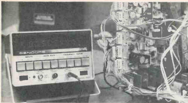
Fig. 8 An accurate counter is needed to check frequencies in any digital circuit, including this check of the master scan oscillator frequency.
