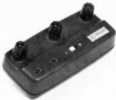
Fig. 2 Design of this current shunt is simple. The input current is fed through a chunk of resistive material and the resulting voltage drops measured. This model can 10 A or 31.6 A. measure
