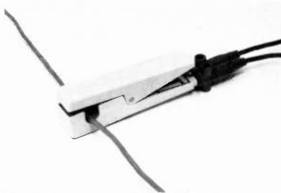
Fig. 3 Modern current transformers are simple clip-on affairs, the small compact design minimizing losses. Maximum reading from this model is around 100 A.
