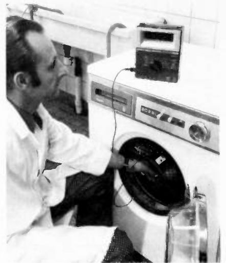
Fig. 7 A temperature measuring capability is useful addition to a multimeter, enabling many measurements to be speeded up—from regular servicing as shown here to electronic circuit troubleshooting.
