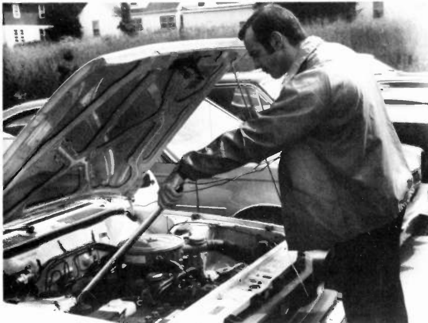
Fig. 9—A new service tool called the Channel Master "Sleuth" (Model 5270) helps pinpoint tough dog noise source.
