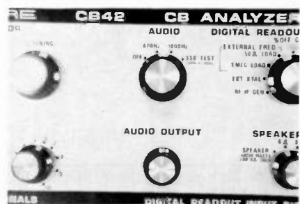
Fig. 6—CB42 audio generator frequency-selector ('AUDIO') and output level ('AUDIO OUTPUT') controls.
