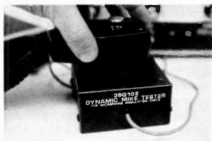
Fig. 7—39G102 Dynamic Mike Tester, shown here being used to feed output of CB42 audio generator directly into mike of CB transceiver.
