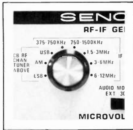
Fig. 3—Eight-position "RF-IF GENERATOR" switch of CB42.
