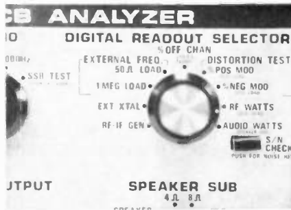
Fig. 2—"DIGITAL READOUT SELECTOR" switch of CB42 determines which CB transceiver characteristic is to be measured and read out by digital display. In addition, "RF-IF" position of switch provides readout of internal generator output frequency.
