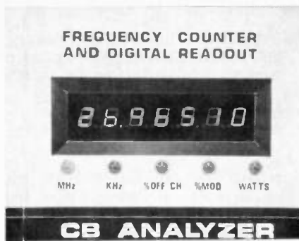
Fig. 1—Auto-ranging, 7-digit, LED digital display provides readout of all CB transceiver characteristics measured by CB42, plus frequencies of RF and IF signals generated by CB42.
