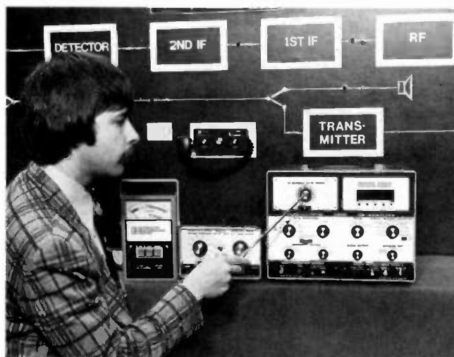
Fig. 1—Greg Carey, Sencore chief field engineer, points to 45-channel RF tuner section of the CB-42 CB Analyzer, which combines a frequency counter, RF/IF generator, audio generator, digital RF wattmeter, and special CB tester, all in one unit for CB servicing. To the left of the analyzer is Sencore's portable power supply/battery eliminator and the CB automatic performance tester.
