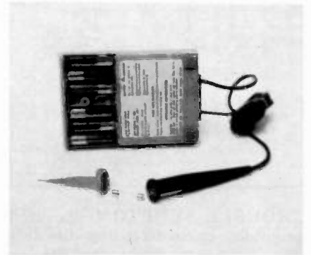
Fig. 2—Rear view of DVM36, with battery compartment cover removed to show battery complement, and tip of 'Touch-On' probe unscrewed from handle to show 2-amp overload protection fuse in probe.
