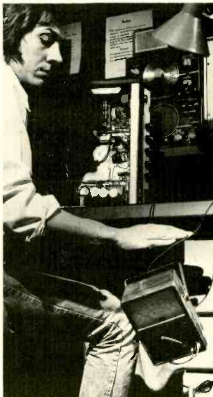
Triplet's Model 60 VOM is shock-resistant to accidental drops up to five feet.
