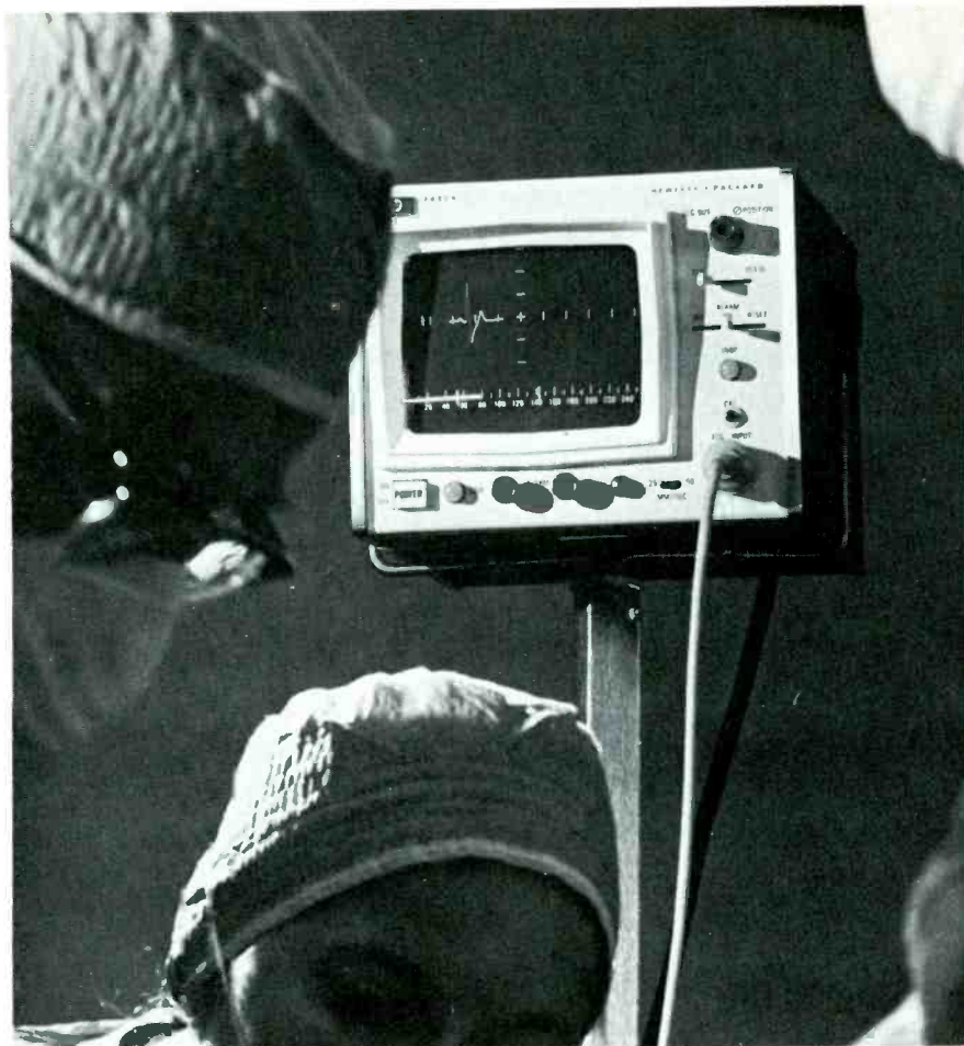
Fig. 5—Self - contained medical monitor system for use in operating rooms, intensive and coronary care facilities and emergency rooms. (Courtesy: Hewlett - Packard.)
