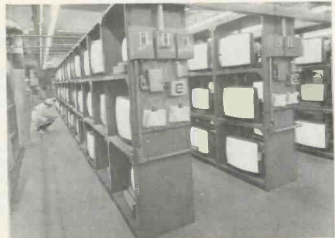
17) A sample from each day's production is put on life test. These tubes are "on" continuously at 10 percent above rated anode voltage and normal line voltage for 5,000 hours. Each tube on life test is monitored daily to insure that it is still operating. Some of these tubes continue to be tested to ultimate life. Normally, 1000 picture tubes are on life test simultaneously. ■
