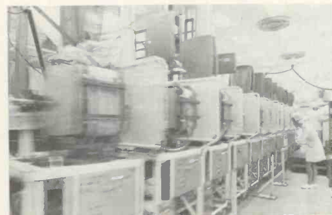
6) The aluminizing equipment shown here puts a reflective surface on the inside of the face panel. The panels are vacuum-sealed in individual frames, and as they proceed through this process, aluminum is evaporated evenly over the entire inside section of the faceplate. After aluminizing, the panels are baked in an oven, to remove any impurities and moisture in the screen and glass.
