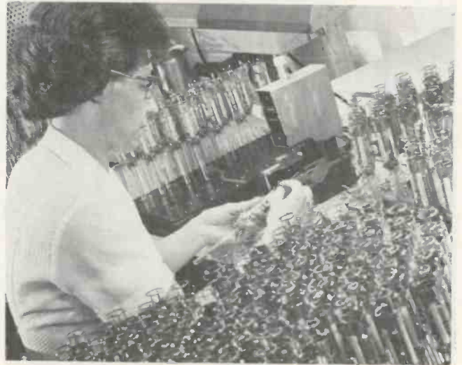
10) In this operation, electron guns are being prepared for mounting in the tubes. The operator is welding "getters" onto the mounts. They receive a liquid nitrogen bath prior to mounting, to remove any particles of lint or weld splatter that may have accumulated.
