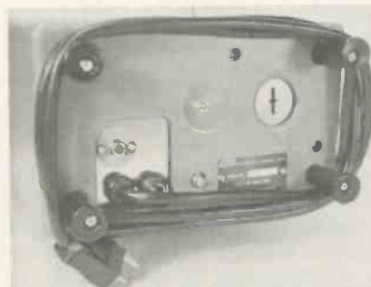
Rear view of the Model 1431. The jack above the line cord input is the Z-AXIS input, which provides intensity modulation for time or frequency marking of the displayed waveform. The line fuse is located beside the line cord input. The circular disc with a long slot is the CRT positioning device, which is described in the text.
