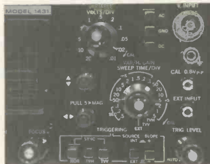
Close-up view of the conveniently grouped vertical, horizontal and sync controls of the Model 1431.
