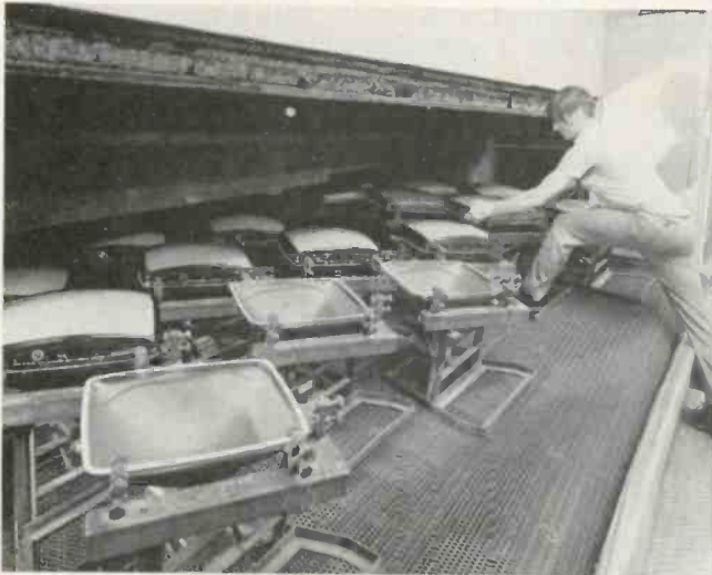
9) After frit application, the funnel and faceplate are joined and travel, for approximately one hour, through an oven at temperatures up to 450° (C). During this operation, the frit is converted to a ceramic-like material, and the resulting bond between panel and funnel is made permanent. The panel and funnel are held in the precisely adjusted fixtures shown here, to insure accurate alignment of the bonded parts.
