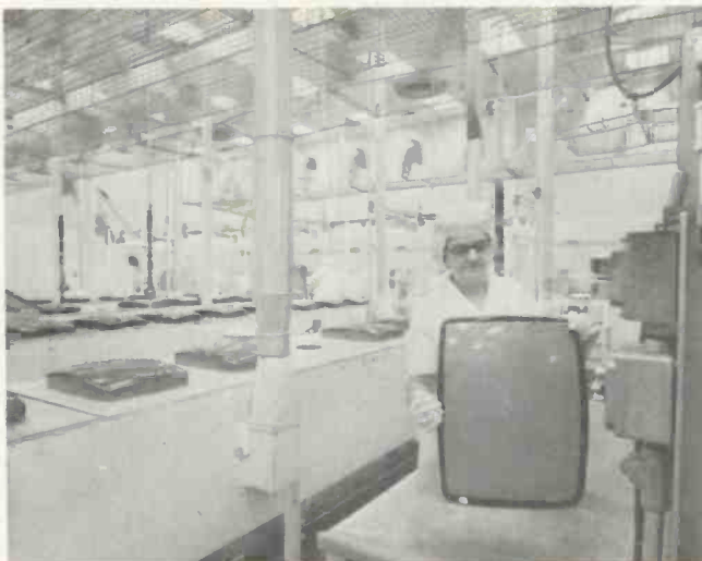
5) An inspector examines a faceplate for any defects. Rejects are carefully examined and recycled.
