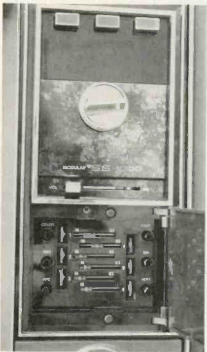
The M25 chassis uses a 12-position VHF tuner and a varactor-tuned UHF tuner. Six thumb-knob adjustments are used to pretune any six UHF channels.
