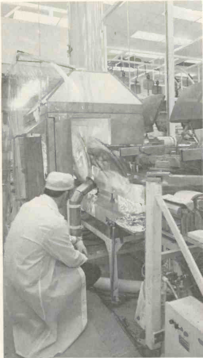
2) In making "Chromatrix" black matrix tubes, before the color phosphor dots are applied, a black material is placed on the face panel. Exposure tables, with similar optical systems, are used to produce holes or windows at the proper locations in the black material. The panel then proceeds to the screening room, where the phosphor dots are applied over their respective windows. The foreman is watching the spinning operation which dries the polyvinyl alcohol on the tube panel before exposure.
