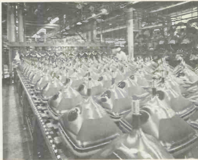
14) An external conductive coating is applied on the tube funnel, to form a capacitor. After this process, the tubes are placed on a huge conveyor, as shown here, and special heaters dry the external conductive coating.
