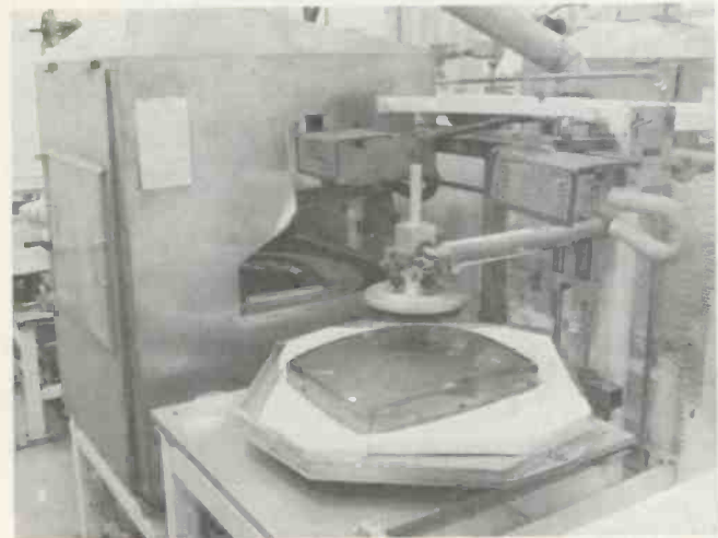
4) The methacrylate lacquer is applied automatically in the booth in the background, while the faceplate is spun to assure even surface distribution. The vacuum chuck removes the lacquered faceplate from the booth and deposits it on the blotting material in the foreground.
