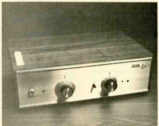
Fig. 4—TOCOM's subscriber terminal.
