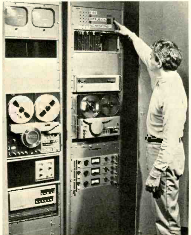
Fig. 3—Community Information System's headend for two-way CATV.
