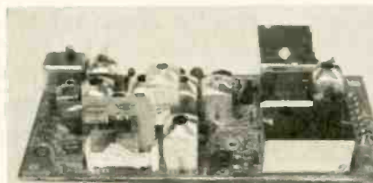
The "A" panel contains the following circuits: AFC, video IF, video detector, video driver, 45.75MHz detector, sound IF and quadrature detector module.
