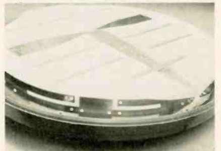
Two angular views of the antenna showing the VHF elements around the perimeter and the UHF elements in the middle.
