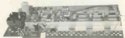
Top view of digital tuning indicator circuitry with lamp assembly removed.
