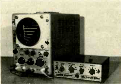
Fig. 1—The Model A curve tracer teams up with a general-purpose scope to become a complete semi-conductor testing facility.
